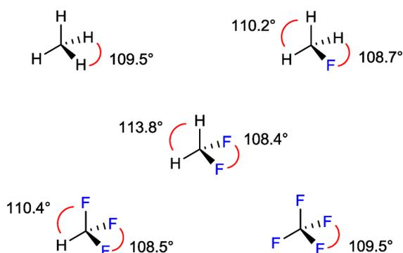
Fig. 3 Bond angles in methane and the fluoromethane series.
