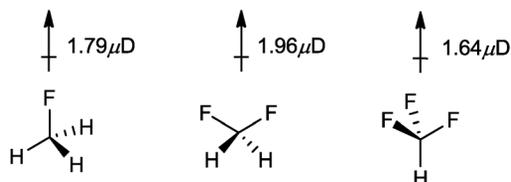
Fig. 4 Dipole moments of fluorinated methanes [14].
