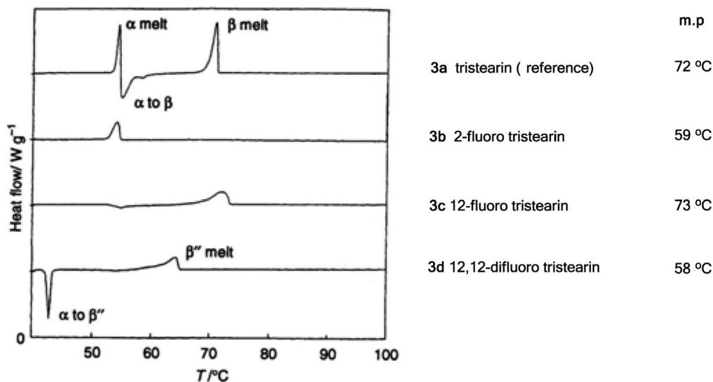
Fig. 10 DSC thermogram of tristearin **3a** and fluorinated tristearins **3b–d** [9].
