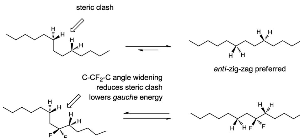
**Fig. 11** CF<sub>2</sub>-functionalized aliphatic chain introduce increased conformational disorder.
