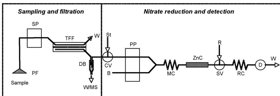
**Fig. 2** Flow analysis manifold used for the determination of nitrate in coastal marine and estuarine waters. PF, prefilter; SP, sampling pump; TFF, tangential flow filter; W, waste line; DB, debubbler; W/MS, waste/manual sampling line; St, standard; CV, calibration valve; PP, peristaltic pump; B, buffer line; MC, mixing coil; ZnC, zinc column; R, Griess reagent; SV, solenoid valve; RC, reaction coil; D, detector. Reprinted with permission from ref. [12]. Copyright © (2011), Elsevier B.V.
