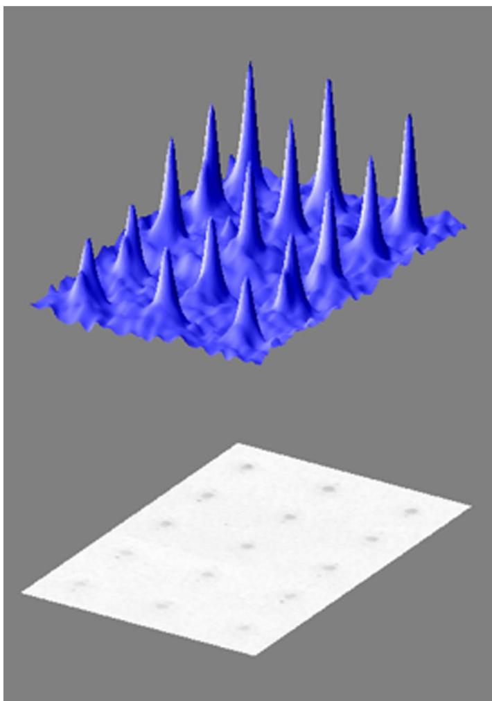
**Fig. 7** Scanned image of a paper-based device after addition of  $0.1\text{--}1.0 \text{ mg P L}^{-1}$  phosphate standards with corresponding 3D densitometric image from which calibration data are obtained.
