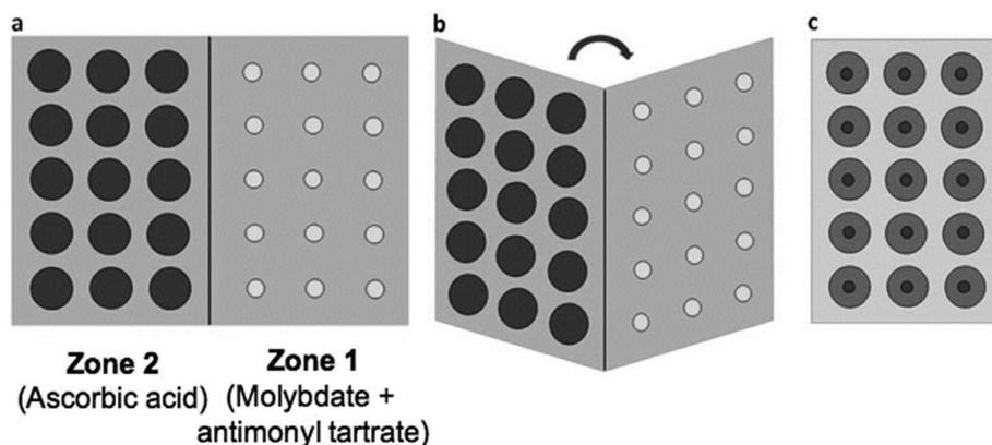
**Fig. 6** Diagram showing the sequence of operations in the preparation of a paper-based device for determination of phosphate: (a) Inkjet-printed paper with reagents applied to zones 1 and 2, (b) paper folded so that centers of zones 1 and 2 align, (c) folded paper laminated and holes punched in laminate to allow sample addition to zone 2.
