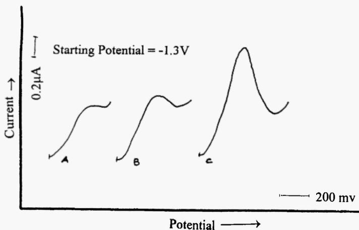
**Fig. 4:** DP polarogram of pyruvic acid in 0.1M  $\text{NH}_4\text{Cl}$  and 0.005M  $\text{NH}_4\text{OH}$  solution at pH 3.1 showing effect of concentration. (A) 1.38 mg, (B) 2.6 mg, (C) 4.4 mg (per 100 ml of analyte).
