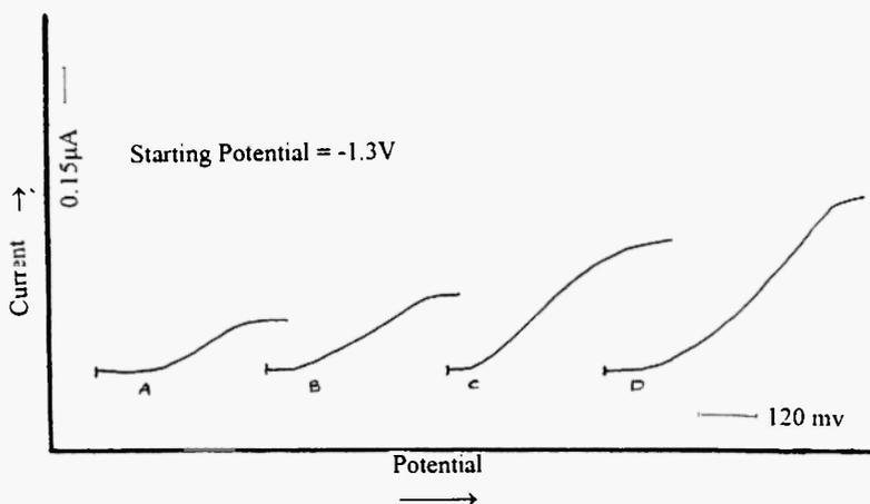
**Fig. 3:** DC polarograms of pyruvic acid in 0.1M  $\text{NH}_4\text{Cl}$  and 0.005M  $\text{NH}_4\text{OH}$  solution showing effect of concentration. (A) 2.2 mg, (B) 4.4 mg, (C) 6.6 mg, (D) 8.8 mg (per 100 ml of analyte).
