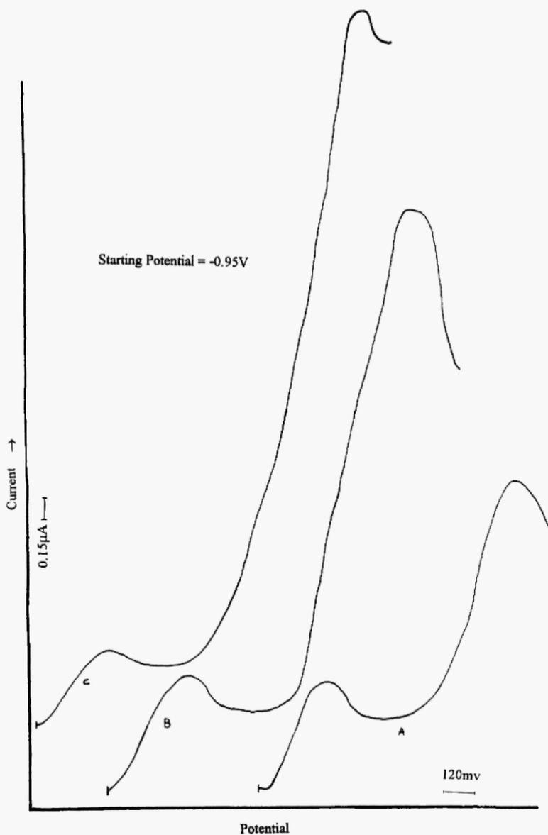
**Fig. 1:** DC polarograms of cystine in 0.1M  $\text{NH}_4\text{OH}$ , 0.1M  $\text{NH}_4\text{Cl}$  and 0.001M  $\text{CoCl}_2$  solution at pH 8.5 showing effect of concentration. (A) 0.24 mg, (B) 0.6 mg, (C) 1.2 mg (per 100 ml of analyte).
