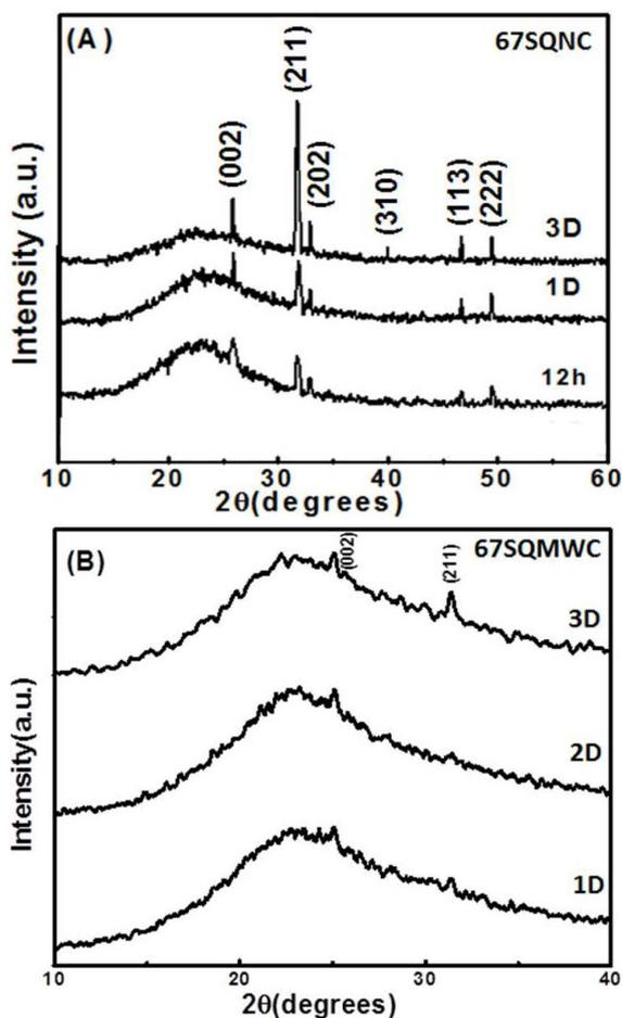
**Figure 5:** XRD pattern of (A) 67SQNC glass soaking in SBF for 12 h, 1D and 3D (B) 67SQMWC glass soaking for 1D, 2D and 3D.
