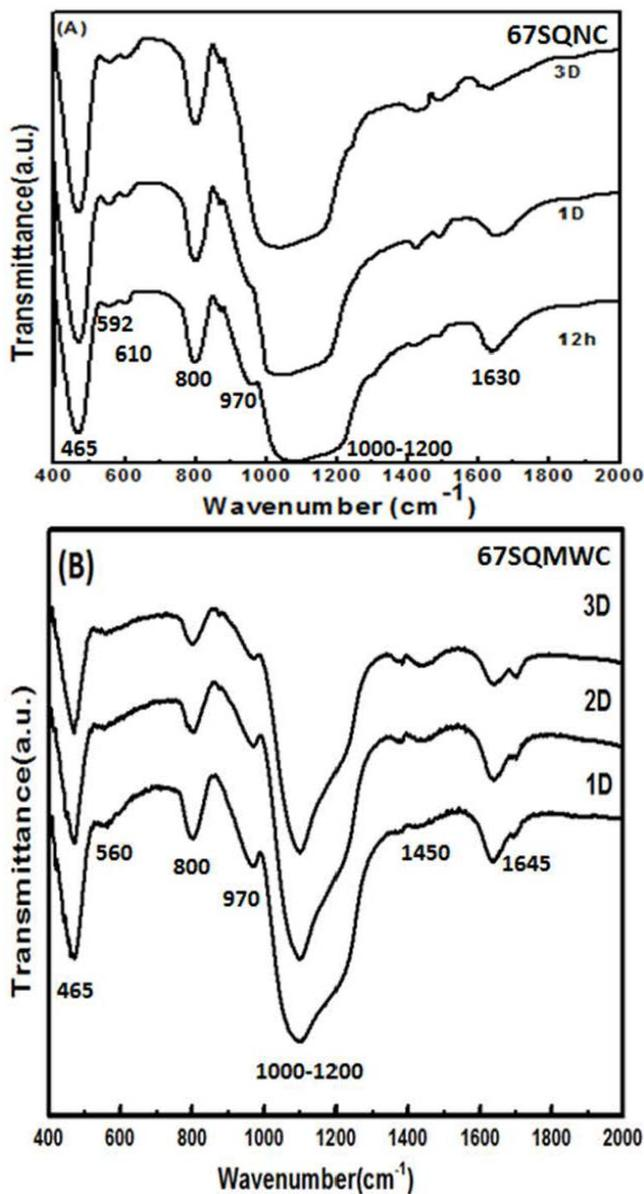
**Figure 6:** FTIR Spectra of (A) 67SQNC glass sample after soaked for 12 hours, 1D and 3D (B) 67SQMWC glass sample after being immersed in SBF for 1D, 2D and 3D.
