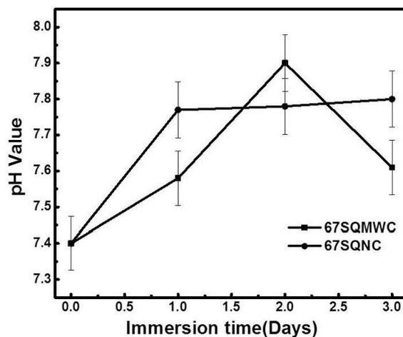
**Figure 4:** The variation of pH values SBF solution as a function of soaking time.
