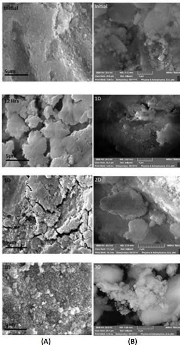
**Figure 7:** (A) SEM micrographs of 67SQNC glass before and after soaking for 12 hours, 1 and 3 days. (B) FESEM micrographs of 67SQMWC glass before and after soaking for 1, 2 and 3 days.
