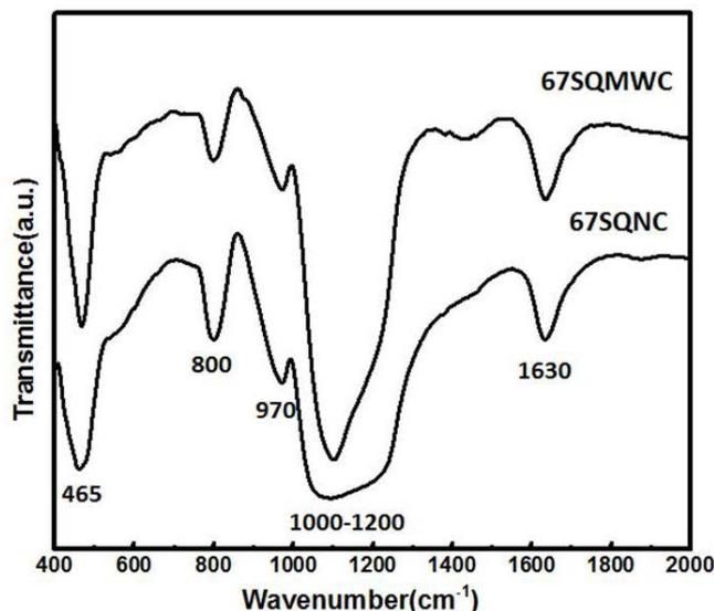
**Figure 1:** FTIR spectra of 67SQNC and 67SQMWC glass sample after the calcination process.
