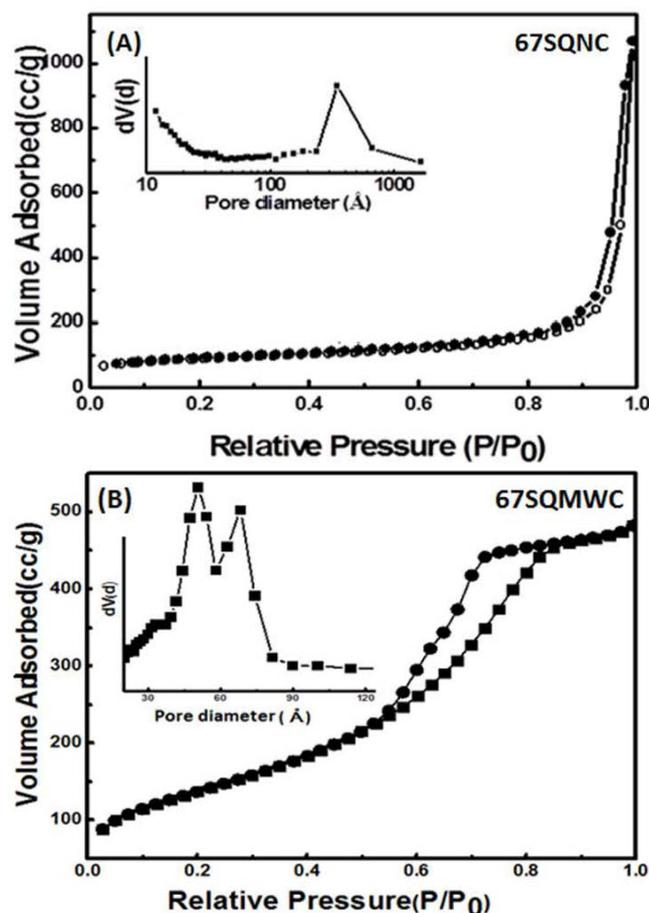
**Figure 2:** Nitrogen adsorption–desorption isotherm and pore size distribution (inset) of (A) 67SQNC (B) 67SQMWC glass samples in their pristine form
