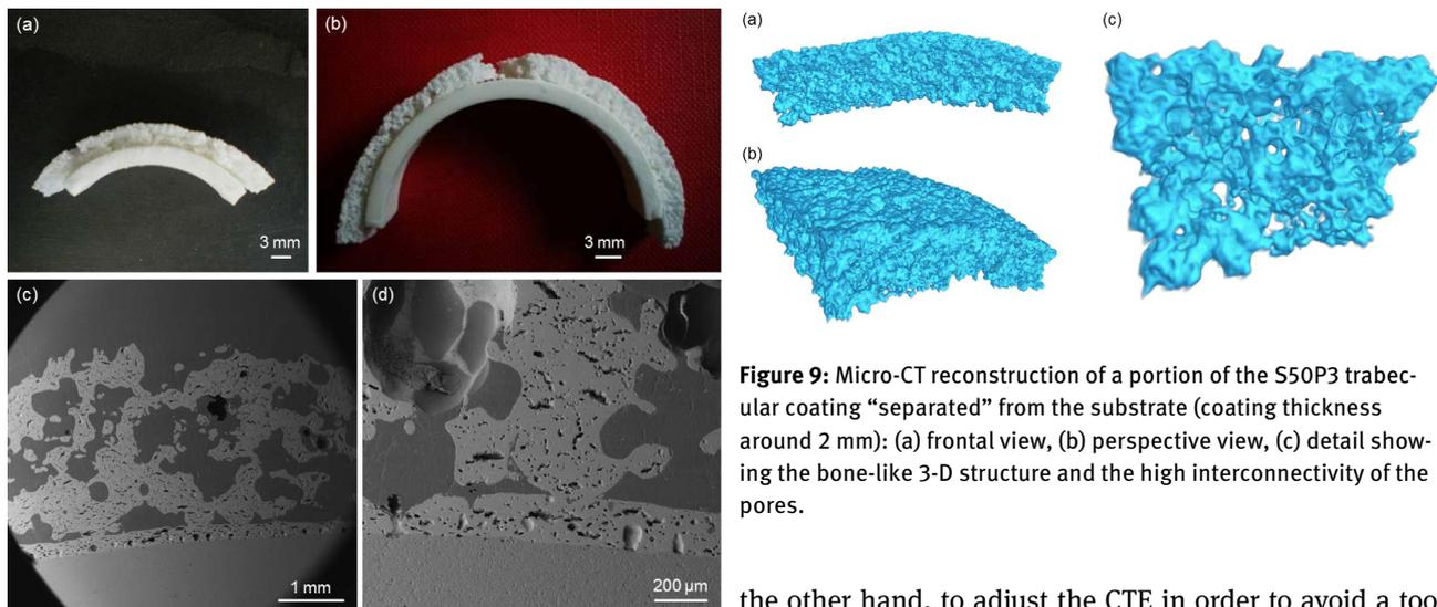
**Figure 8:** Complete curved samples (alumina substrate + SCNA interlayer + S50P3 trabecular coating) after sintering at 1000°C for 3 h: camera pictures of (a) small-sized and (b) large-sized samples; (c) SEM micrograph (back-scattering mode) of a polished cross-section after embedding the sample in epoxy resin (50×) and (d) detail of a contact area between interlayer and trabecular coating (200×).
