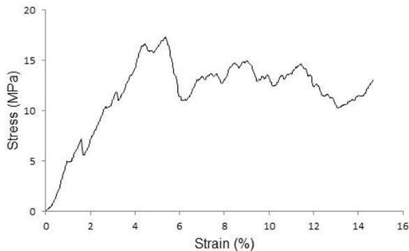
**Figure 6:** Typical stress-strain curve for S50P3 cubic scaffolds.
