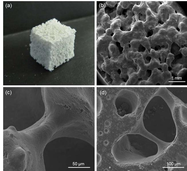
**Figure 5:** Morphological investigation of S50P3 scaffolds: (a) camera picture of a typical porous cuboid (side around 10 mm); SEM micrographs of (b) scaffold surface (magnification 50 $\times$ ), (c) a well-sintered trabecula (1200 $\times$ ) and (d) cross-section showing the interconnectivity of the pores (600 $\times$ ).
