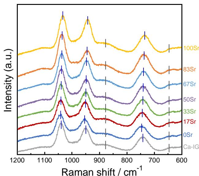
**Figure 2:** Raman spectra of the ySr glasses.
