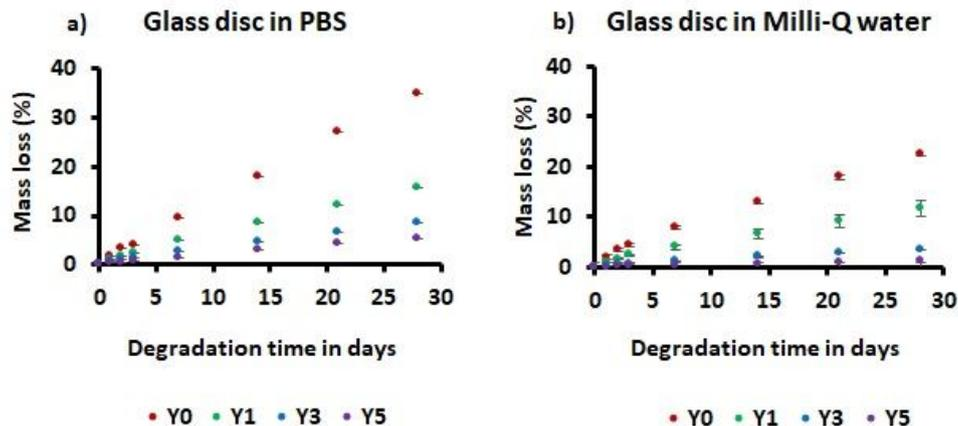
**Figure 7:** Dissolution study for the  $45\text{P}_2\text{O}_5-(30-x)\text{Na}_2\text{O}-25\text{CaO}-x\text{Y}_2\text{O}_3$  (where  $x = 0, 1, 3$  and  $5$ ) glass system conducted in (a) PBS and (b) Milli-Q water at  $37^\circ\text{C}$
