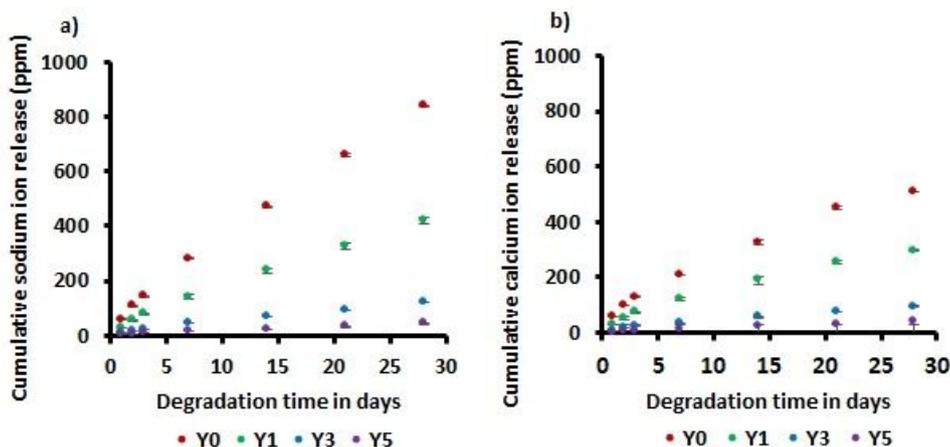
**Figure 9:** Cumulative ion release profile of glass discs at different glass formulation in Milli-Q water for 28 days a) Sodium ion release and b) Calcium ion release. (Error bars are also included in the data above)
