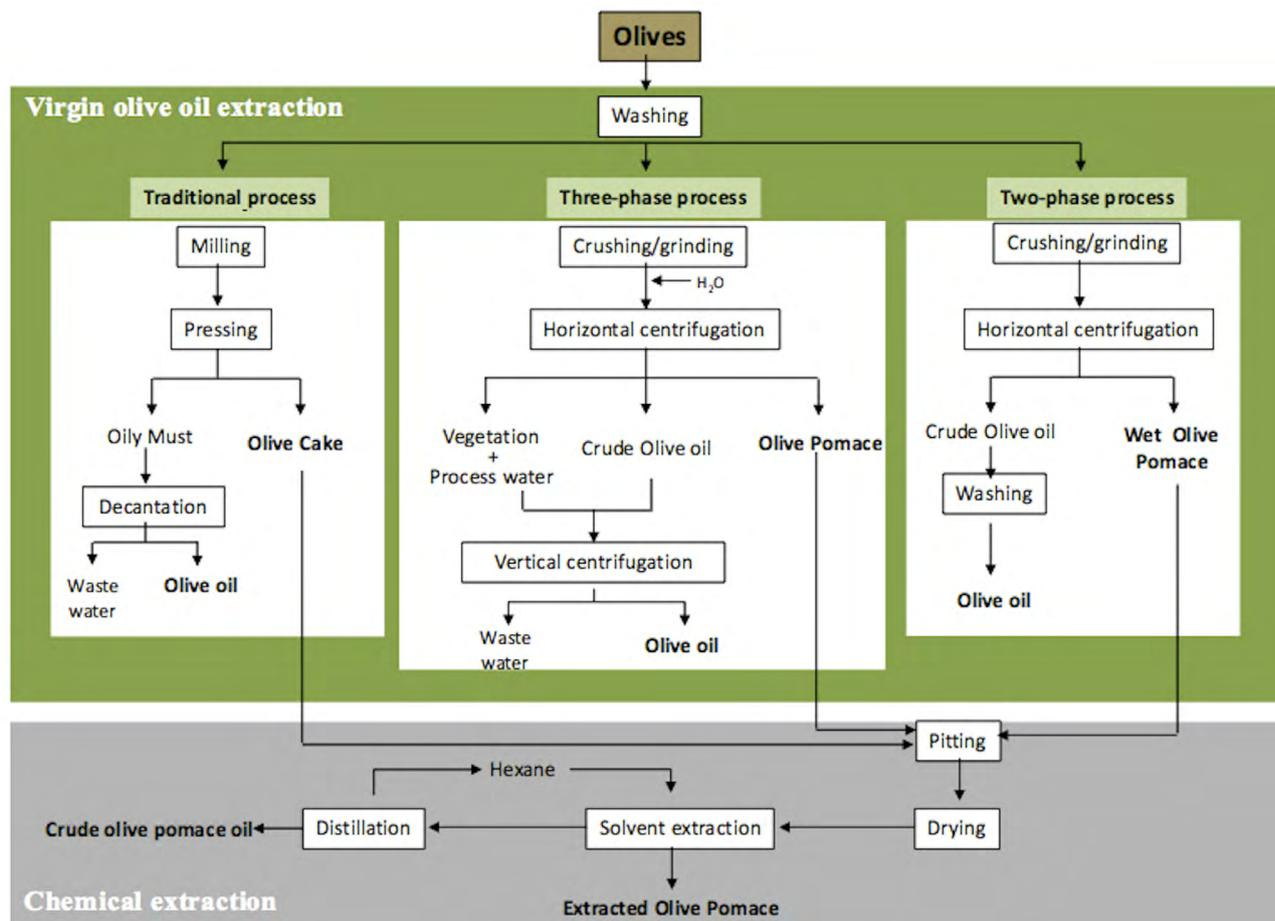
**Figure 1:** Different methods of olive oil and olive pomace oil extraction and their products and by-products.
