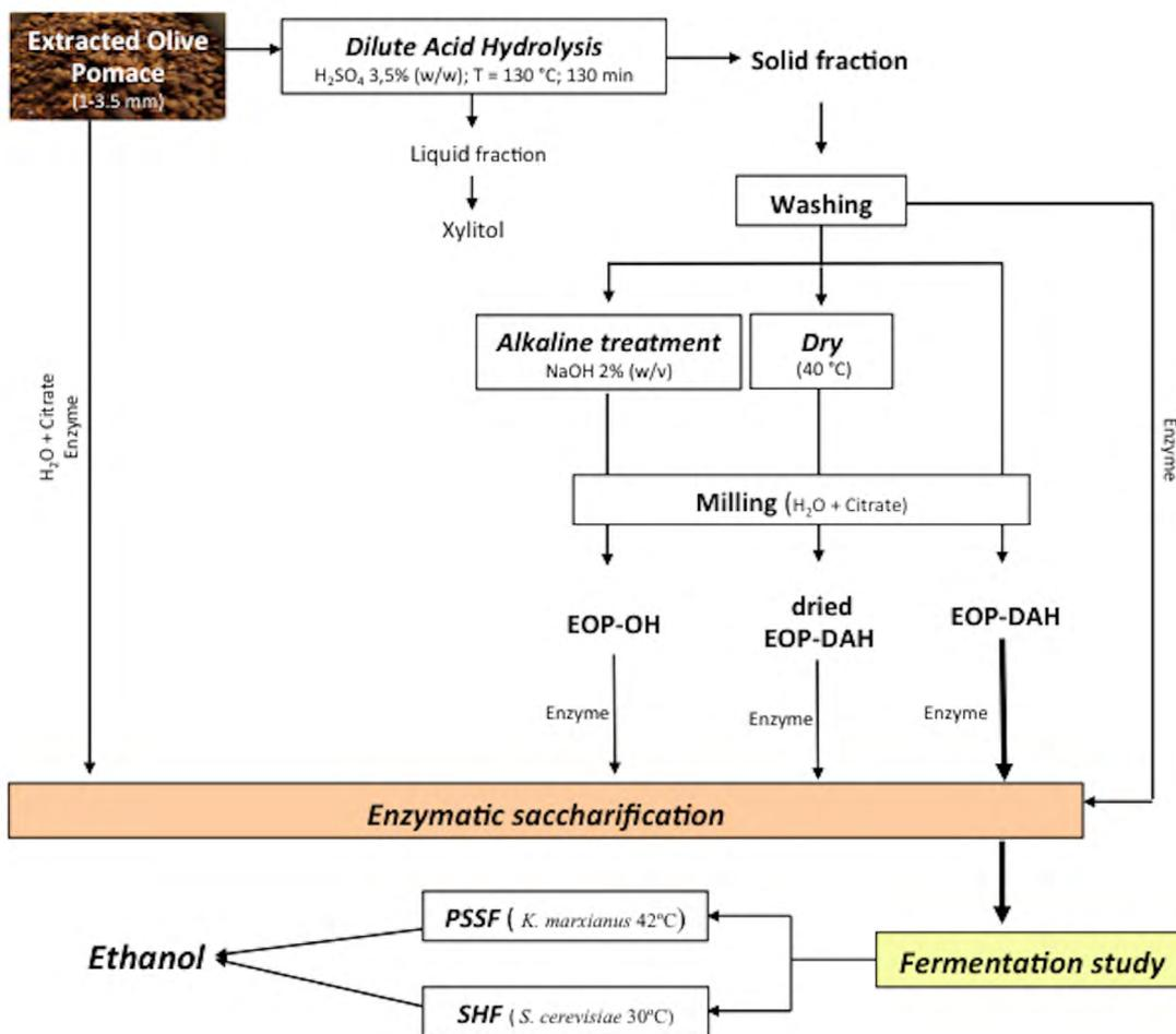
Figure 2: Schematic representation of biomass pretreatment, enzymatic hydrolysis and fermentation process.
