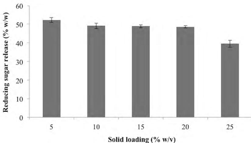
**Figure 3.** Effect of solid loading (% w/v) on reducing sugar release at constant conditions (Reaction time: 10 min;  $H_2SO_4$ :1.5% v/v; Temperature: 120°C (under 100 kPa pressure)).
