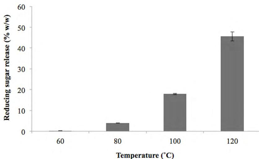
**Figure 1.** Effect of temperatures ( $60^\circ C$ ,  $80^\circ C$ ,  $100^\circ C$  in water bath and  $120^\circ C$  in autoclave at 100 kPa) on reducing sugar release at constant conditions (Reaction time: 10 min; Solid load: 5% w/v;  $H_2SO_4$ :1% v/v).
