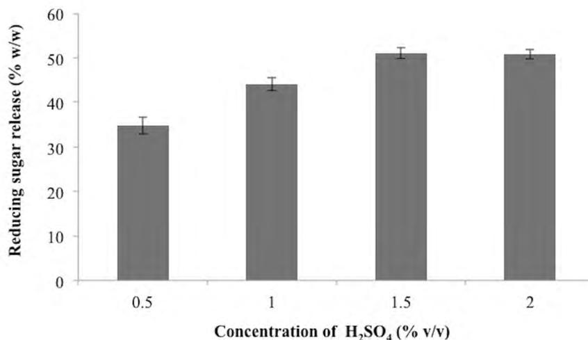
**Figure 2.** Effect of  $H_2SO_4$  Concentrations (% v/v) on reducing sugar release at constant conditions (Reaction time: 10 min; Solid load: 5% w/v; Temperature:  $120^\circ C$  (under 100 kPa pressure)).
