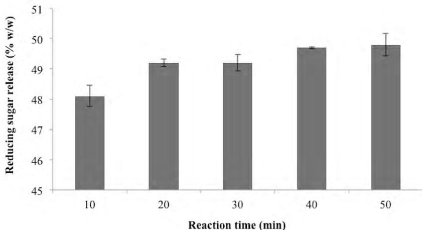
**Figure 4.** Effect of reaction time (min) on reducing sugar release at constant conditions (Solid load: 20% w/w;  $H_2SO_4$ :1.5% v/v; Temperature: 120°C (under 100 kPa pressure)).
