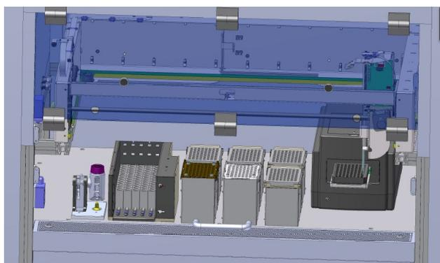
**Image 1** Diagnostics platform for personalized chemosensitivity assays (CAD front view)
