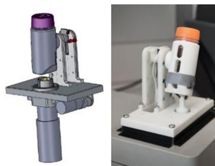
**Image 2** First prototype of tissue processing unit with integrated heating device
