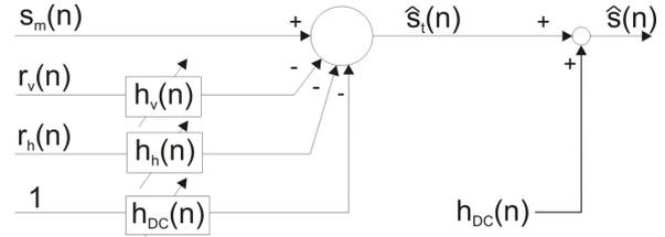
Figure 1: Adaptive filter structure
