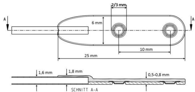
Figure 1: Schematic drawing of the developed silicone electrode for subepimysial implantation.
