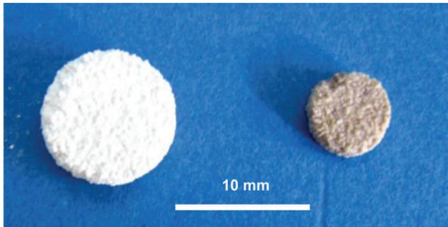
**Figure 2:** Green part and sintered part of M1.
