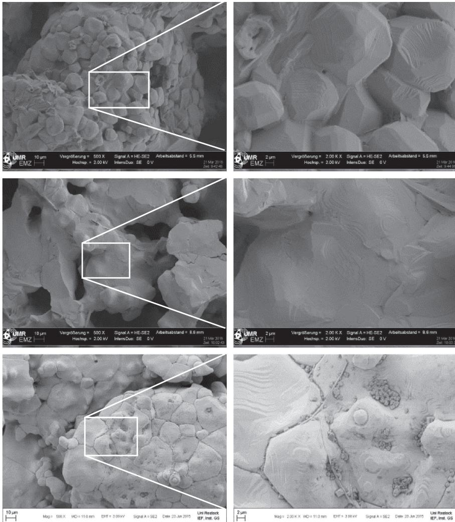
Figure 3: Low (500 ×) and high (2000 ×) magnification of the sintered parts of M1 (top); M2 (middle); M3 (bottom).
