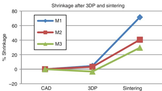
Figure 4: Percentage of shrinkage after 3DP and sintering.
