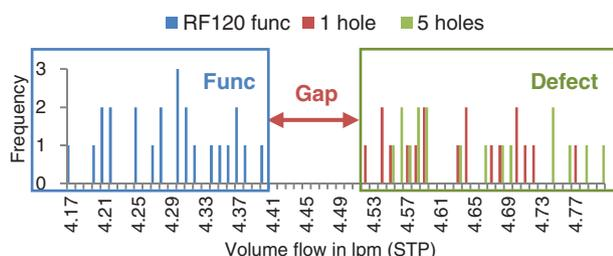
Figure 7: Histogram of 59 RF120 at 500 mbar; argon.
