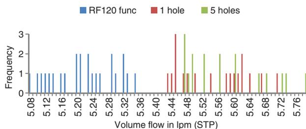
Figure 8: Histogram of 59 RF120 at 500 mbar; nitrogen.
