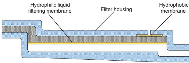
Figure 1: Longitudinal-section of the infusion filter system.
