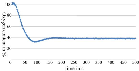
**Figure 5:** time behavior of the oxygen level inside the media using a PID controller
