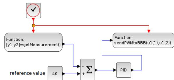
**Figure 4:** Scilab model with PID controller and connection interface to the controlling unit
