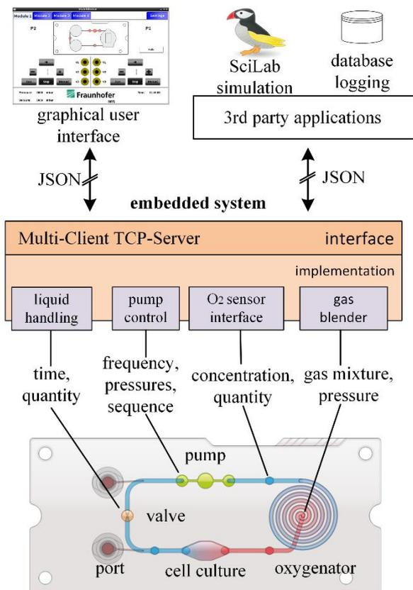
**Figure 2:** software schema of the controlling unit
