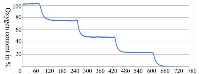
**Figure 3:** stepwise deoxygenation of the process gas stream inside the oxygenator element
