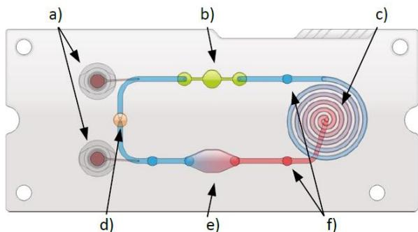
**Figure 1:** MPS layout: a) fluidic ports; b) micro pump; c) oxygenator; f) sensor spots; e) cell culture chamber; d) media exchange valve
