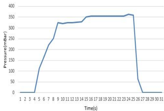
Figure 3: Air Pressure profile applied during flexible probe implantation.
