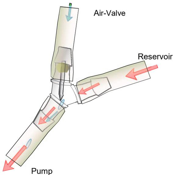
**Figure 1:** Y-connector used for the injection of gas bubbles to the circulation
