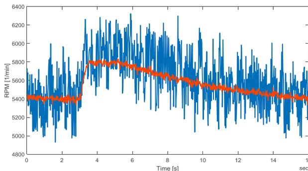
**Figure 4:** Rotational speed diagram whilst the automatic injection of 0.3 ml of air at  $t = 2$  s and the median signal over all measurements
