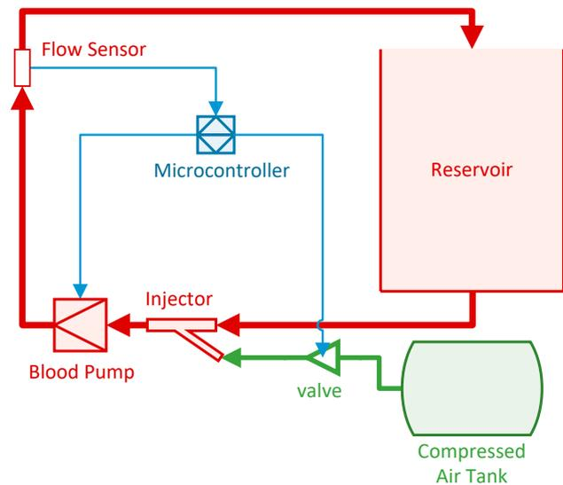
**Figure 2:** Schematic of the presented mock loop
