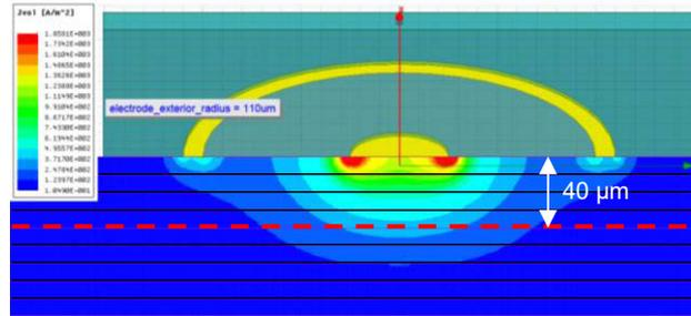
**Figure 2:** Distribution of the current density in the retinal tissue below the electrodes (dark blue colour:  $0.105 A/m^2$ ; dark red colour:  $1.858 kA/m^2$ ). Inner electrode with radius  $25 \mu m$  and outer electrode with radius  $110 \mu m$ .
