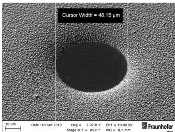
**Figure 5:** Scanning electron microscope images of RIE-etched via hole (diameter: 48  $\mu\text{m}$ ) in a thin polyimide layer. The rounded edges of the polyimide are clearly visible.
