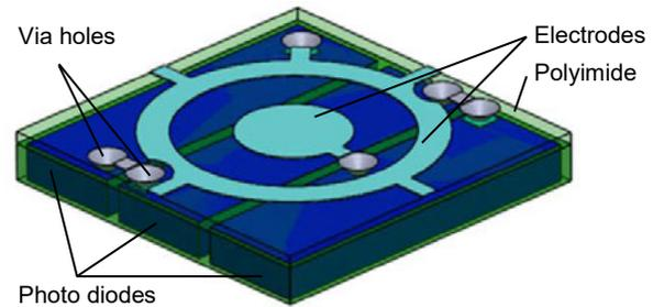
**Figure 1:** Oblique view of one pixel being composed of three photo diodes and separated by 30  $\mu\text{m}$  wide gaps. A thin layer of polyimide spans over all photo diodes. Electrodes are located on top of the polyimide layer. Via holes in the polyimide are required for connecting three photodiodes in series and for connecting electrodes to photo diodes.
