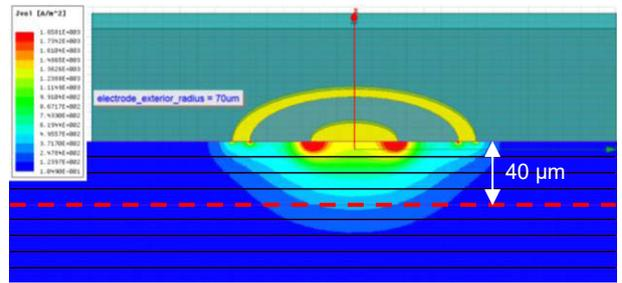
**Figure 3:** Distribution of the current density in the retinal tissue below the electrodes (dark blue colour:  $0.105 A/m^2$ ; dark red colour:  $1.858 kA/m^2$ ). Inner electrode with radius  $25 \mu m$  and outer electrode with radius  $70 \mu m$ .
