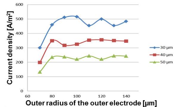
**Figure 4:** The three curves show the simulated maximum current densities below the inner electrode at distances of 30, 40 and  $50 \mu m$  from the plane of the electrodes.
