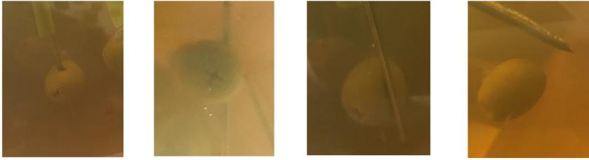
**Figure 3:** Photographs of olive punctured centrally, eccentrically (penetrating flesh or penetrating shell), and olive missed.
