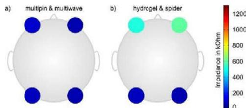
**Figure 2:** Topographic distribution of the electrode-skin impedance before the EEG recordings, calculated over all 10 subjects: a) the hybrid headband equipped with multiwave and multipin electrodes b) the neoprene-only headband equipped with hydrogel and spider-shape electrodes.
