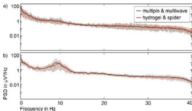
**Figure 3:** Power spectral density of EEG recordings of 30 sec length with a) eyes open and b) eyes closed, averaged over all 10 subjects. Solid lines indicate mean, transparent areas indicate standard deviation.
