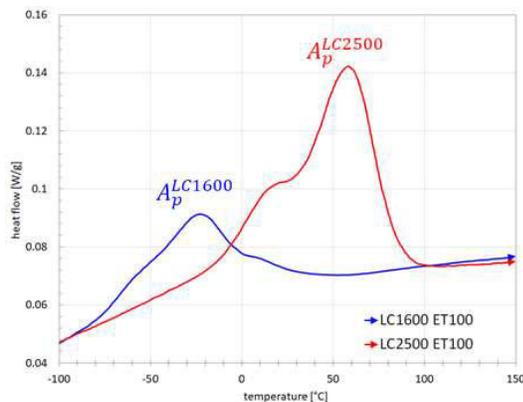
**Figure 5:** DSC heating curves from both sides of the twin-helix produced with specific SLM process parameters Laser Current (LC)  $LC1600$  and  $LC2500$ .
