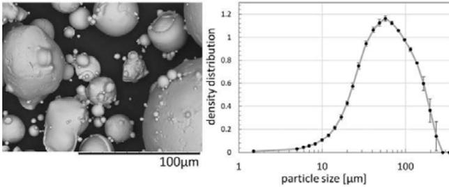
**Figure 3:** a) SEM image and b) particle size distribution of the starting NiTi powder ( $n = 3$ ).
