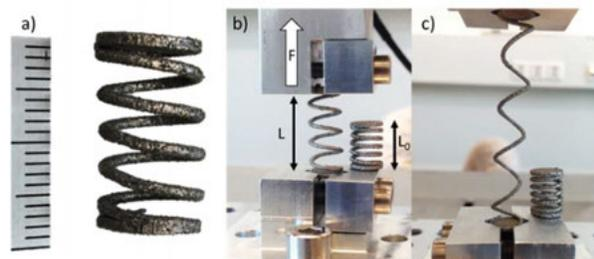
**Figure 1:** a) NiTi helix (scale with millimeter graduation), b, c) during tensile testing. A reference sample is next to it.
