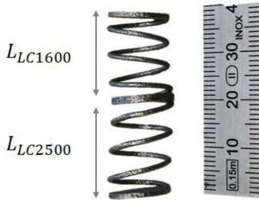
**Figure 2:** Smart twin-helix ( $L_0 = 40$  mm,  $\phi 15$  mm) produced using different SLM parameters *Laser Current* ( $LC$ ).
