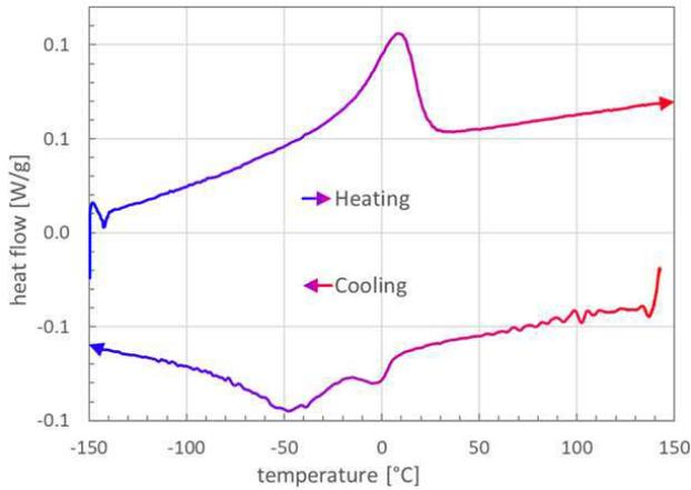
**Figure 4:** DSC curves of the starting NiTi powder.
