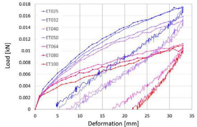
**Figure 6:** Loading and unloading curves of samples produced with specific SLM parameters  $ET025 - ET100$ .
