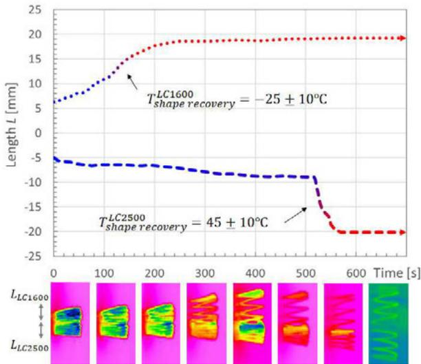
**Figure 8:** a) Temperature-induced shape-recovery and shape-memory phase transformation from *martensite* to *austenite* during warming up. b) Thermograms taken at different stages.
