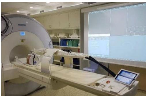
**Figure 3:** Demo setup at PET/MRI (Siemens 3T). Pneumatic robotic arm with attached needle-guide over an abdominal phantom. At the foot end of the patient table are the mouse and the mounted tablet that displays the *Innomotion* control software. In the background the PET/MRI console GUI is projected on the roll screen.
