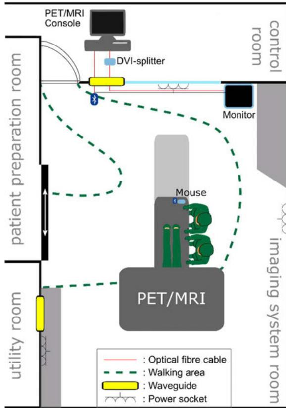
**Figure 1:** Schematic floor plan of the PET-MRI at the Department of Nuclear Medicine at the University Hospital Leipzig (not in scale). Cupboards and shelves depicted in gray in the lower left and upper right corner. Patient entry is possible via preparation or control room.
