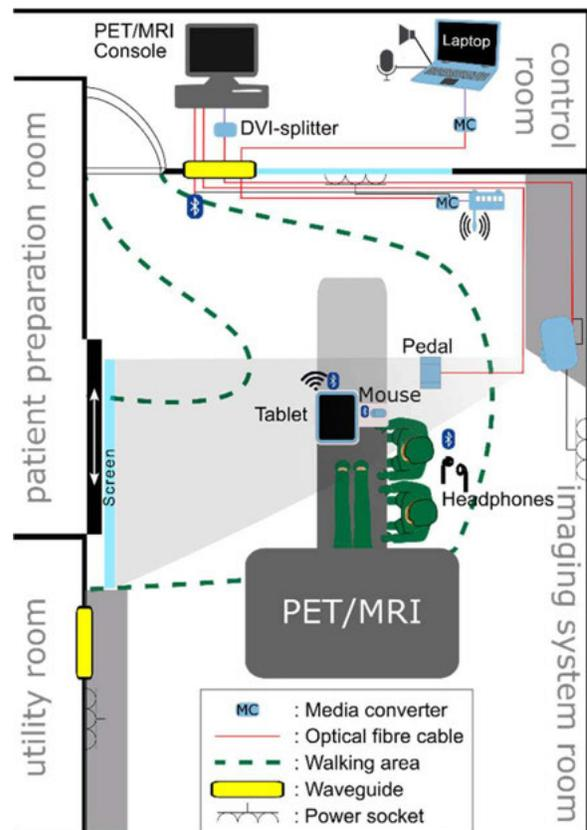
**Figure 2:** The advanced setup comprises multiple input devices, an output device, in-room network for VoIP and/or VNC connection. Although this scheme look overcrowded this it is actually quite comfortable in practical use.
