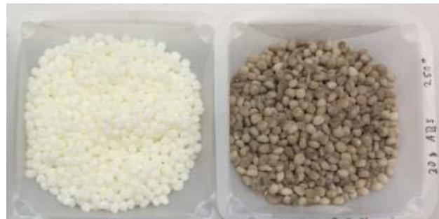
Figure 4: Examples of insufficient mixtures of antimicrobial substance and plastic granulate
