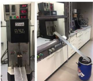
Figure 2: Microcompounder from DACA with metal rail
