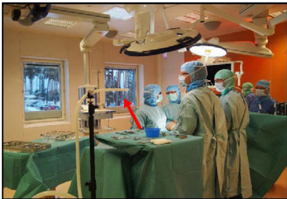
Figure 1: Set-up for the measurement of bacterial air burden with the active air sampling procedure (red arrows indicate the tube-tip for air sampling)
