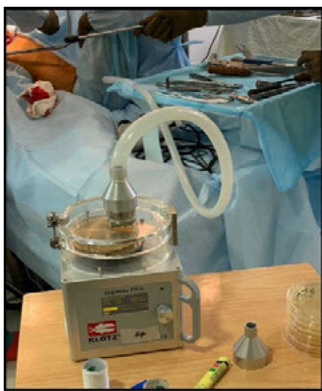
Figure 2: Klotz Impactor FH6 for active air sampling
