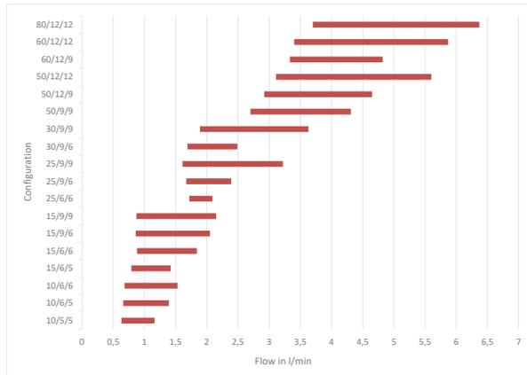
Fig. 3: Blood flow ranges for all pump cannula combinations
