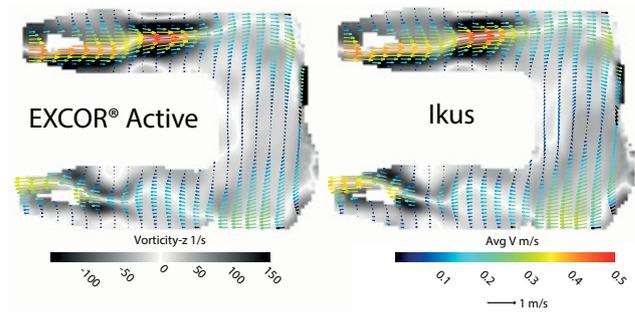
Fig. 5: PIV results for the new EXCOR® Active and the established Ikus driving unit. Vorticity and velocity are averaged over the pump cycle.
