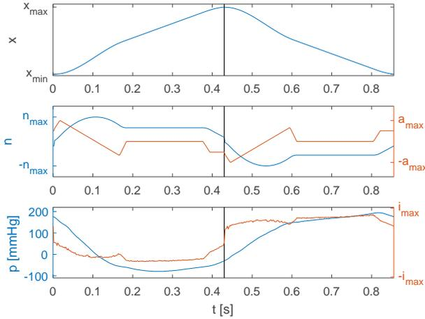
**Fig. 2:** Optimized trajectory for the piston movement: position  $x$  (top), speed  $v$  and acceleration  $a$  (center), relative air pressure  $p$  and motor current  $i$  (bottom)
