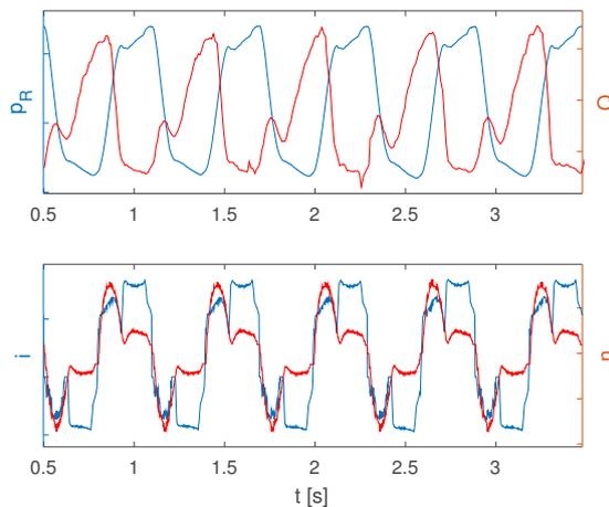
Fig. 4: Logging data for the left 30-ml-pump of a bi-ventricular support patient at a rate of 100 bpm. Drive-line pressure ( $p_R$ ), blood flow ( $Q$ ), motor current ( $i$ ) and piston speed ( $n$ )
