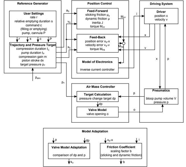
**Fig. 1:** Architecture of the implemented controllers.  $i$ : current,  $p$ : relative pressure,  $a_s$ : reference acceleration,  $v_s$ : reference speed,  $x_s$ : reference position.
