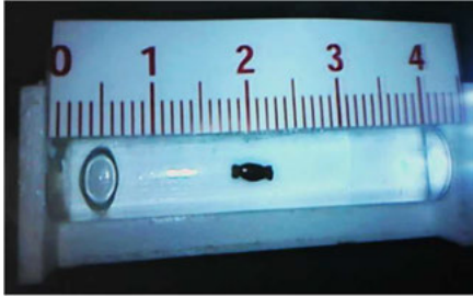
Figure 1: A video still of the swimmer inside the glass tube which is filled with a glycerol-water-mixture. The setup is positioned in the center of the MPI scanner bore. The camera position is below the setup. (The picture is mirrored here, because an endoscopic camera with an attached mirror was used for recording).
