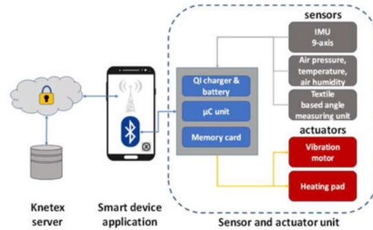
Figure 2: Block diagram of the sensor and actuator system
