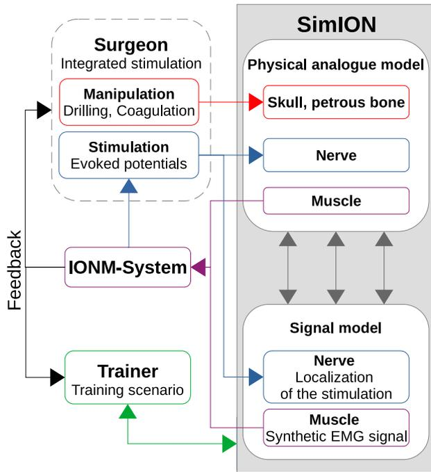
Fig. 2: Schematic structure of the SimION model
