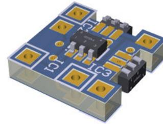
Fig. 3: Single Hall effect sensor module
