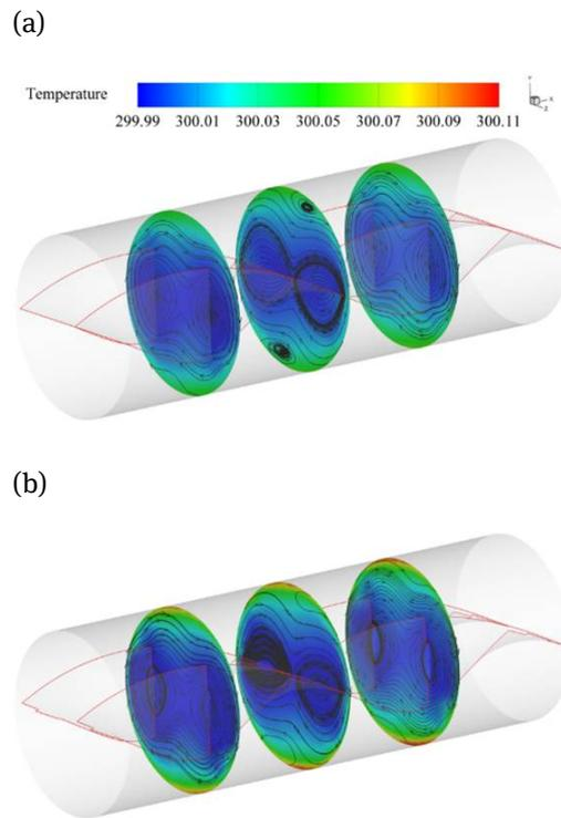
**Figure 5:** Streamline and fluid temperature in cross-section view of tapes: (a) dual twisted tapes (DTs); (b) peripherally-cut dual twisted tapes (PDTs:  $l/y = 0.5$ ).
