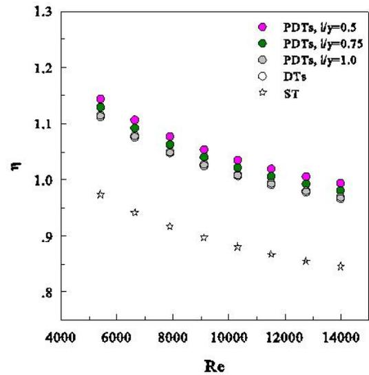
Figure 9: Thermal performance factor against Reynolds number for PDTs at various cutting pitchratios ( $l/y = 0.5, 0.75$  and  $1.0$ ).
