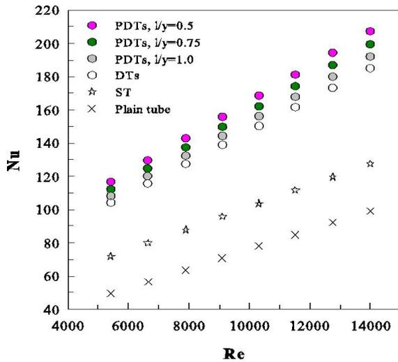
**Figure 4:** Nusselt number against Reynolds number for PDTs at various cutting pitch ratios ( $l/y = 0.5, 0.75$  and  $1.0$ ).
