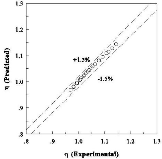
Figure 12: Comparison between predicted and experimental thermal performance factors.
