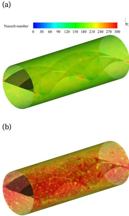
**Figure 7:** Distribution of local Nusselt number around the tube: (a) dual twisted tapes (DTs); (b) peripherally-cut dual twisted tapes (PDTs:  $l/y = 0.5$ ).
