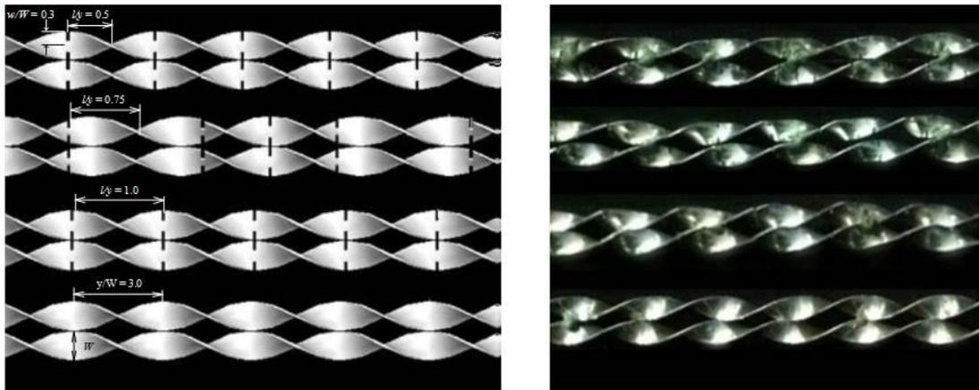
Figure 1: Dimensional parameters and photographs of peripherally-cut dual twisted tapes (PDTs) and dual twisted tapes (DTs).
