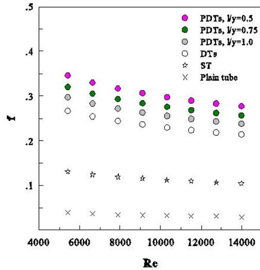
**Figure 8:** Friction factor against Reynolds number for PDTs at various cutting pitch ratios ( $l/y = 0.5, 0.75$  and  $1.0$ ).
