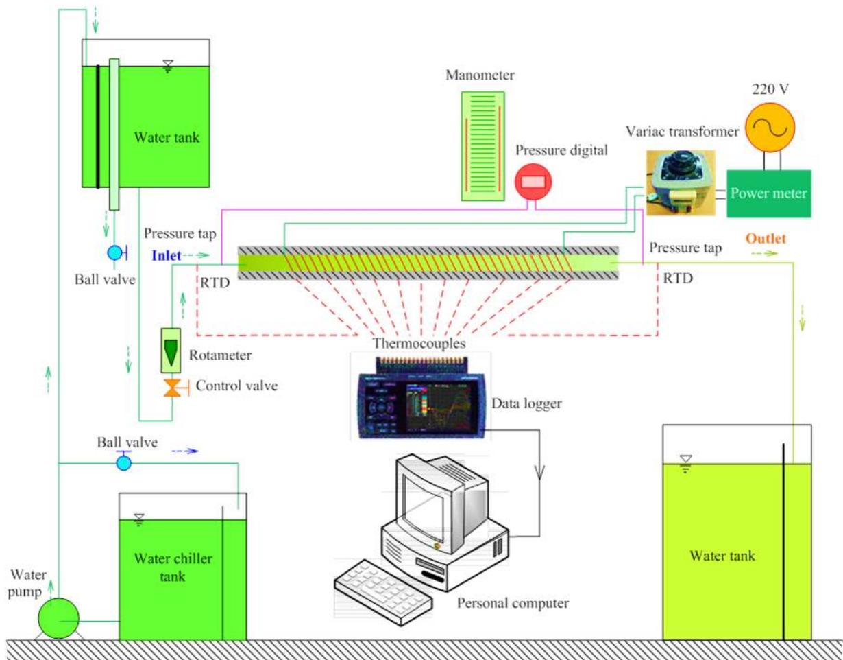
Figure 2: Experimental heat transfer set-up.
