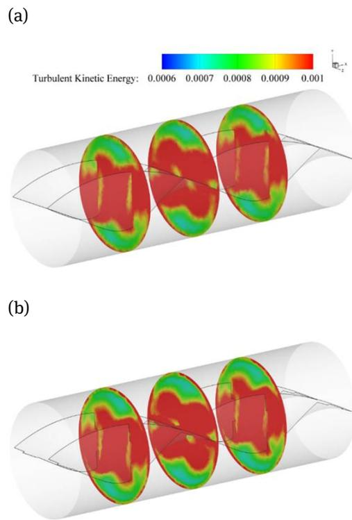
**Figure 6:** Turbulent kinetic energy (TKE) in cross-section view of tapes: (a) dual twisted tapes (DTs); (b) peripherally-cut dual twisted tapes (PDTs:  $l/y = 0.5$ ).
