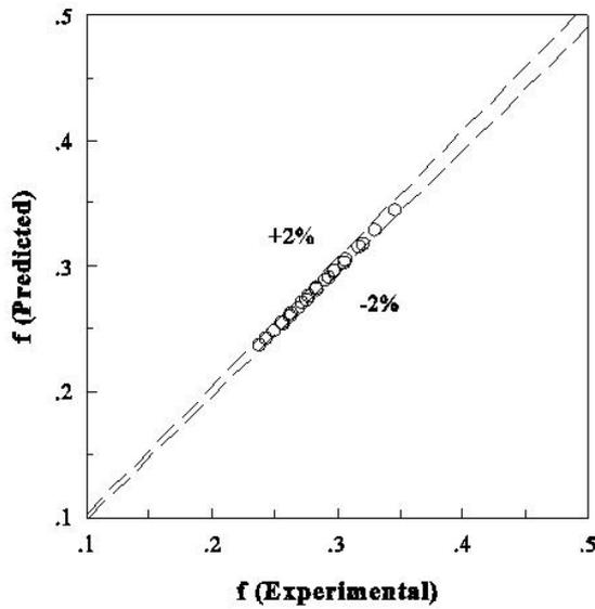
Figure 11: Comparison between predicted and experimental friction factors.
