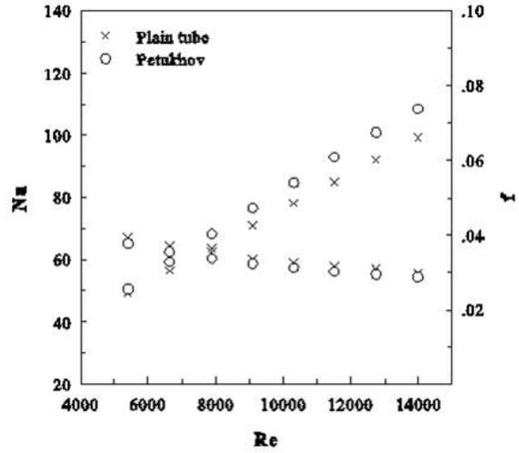
**Figure 3:** Data verification of mean Nusselt number and friction coefficient for the plain tube.
