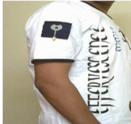
Figure 8: Proposed antenna while measuring results on vector network analyser in IIT Kanpur lab.
