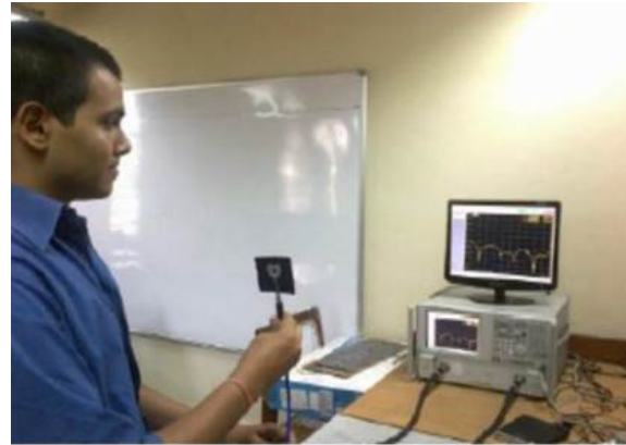
Figure 8: Proposed antenna while measuring results on vector network analyser in IIT Kanpur lab.
