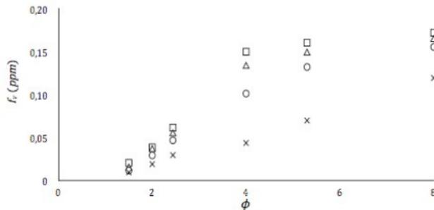
**Figure 3:** Relationship between the  $f_v$  formed for each  $\phi$  used. The following symbols represent the measuring height from the base of the flame: (x) of 5 mm, (o) of 10 mm, ( $\Delta$ ) of 15 mm and ( $\square$ ) of 20 mm.
