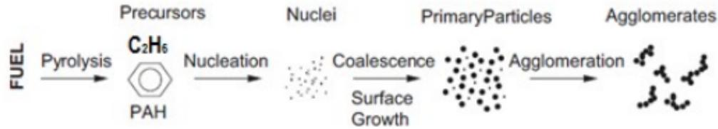
Figure 1: Stages of the soot formation process [13].
