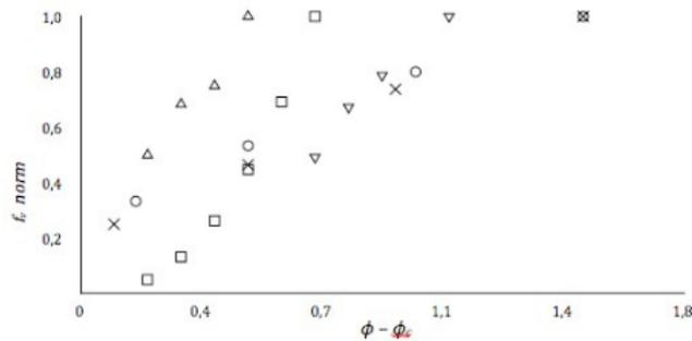
**Figure 4:** Normalized  $f_v$  values in function of the equivalence ratio ( $\phi - \phi_c$ ) for the present study (x), in comparison to the results of [12], ( $\Delta$ ), [17] ( $\square$ ), [19] ( $\nabla$ ) and [18] (o).
