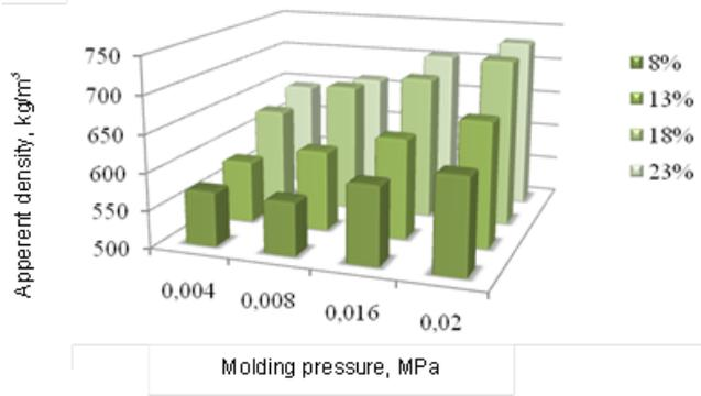
**Figure 1:** Variation in apparent density with molding pressure and content of polymer binder (8, 13, 18 and 23 wt.%).
