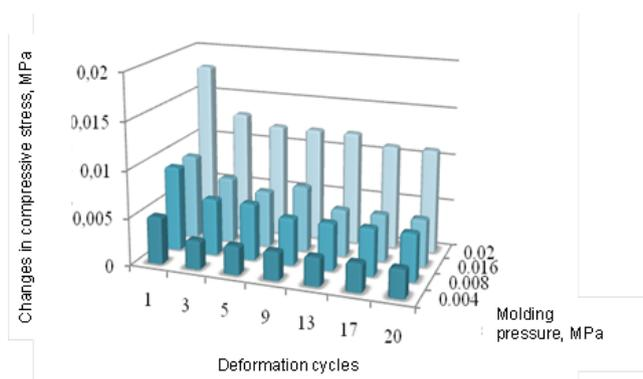
**Figure 3:** Changes in compressive stress at 10% deformation with number of deformation cycles of composite material and molding pressure. Polymer binder content 18 wt.%
