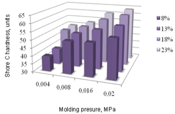
**Figure 2:** Shore C hardness dependence on molding pressure and content of polymer binder (8, 13, 18 and 23 wt.%).
