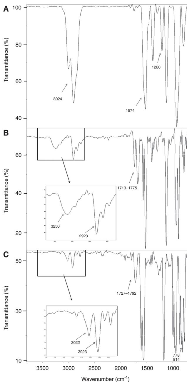
**Figure 2** The FTIR spectra of (A) MPS-Cl, (B) MPS TET, and (C) MPS TET-Cl.
