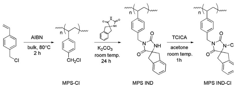
**Figure 1** Scheme of the synthesis of *N*-halamine hydantoin-containing polystyrenes.
