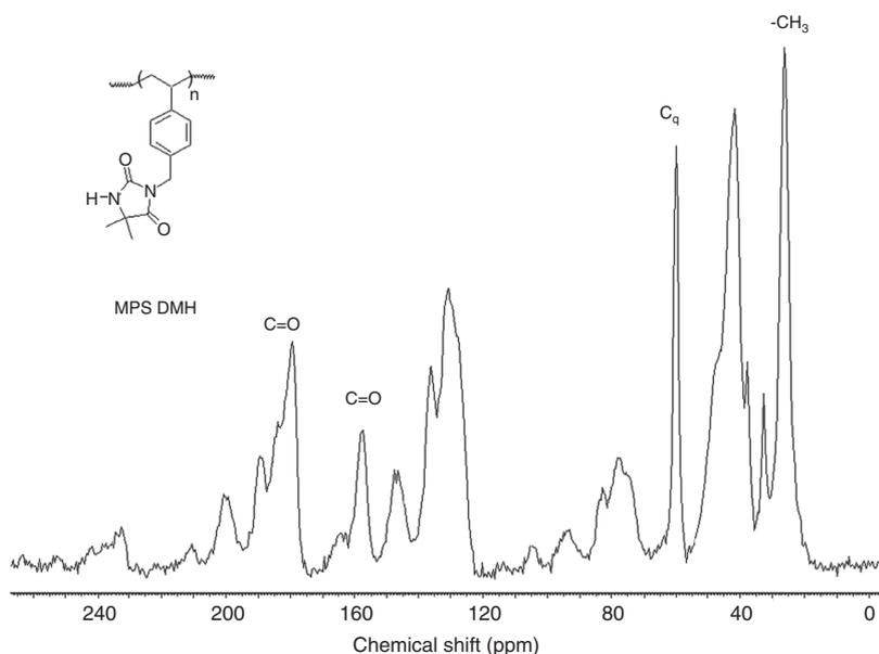
**Figure 3** Solid-state  $^{13}\text{C}$  NMR spectrum of MPS DMH.
