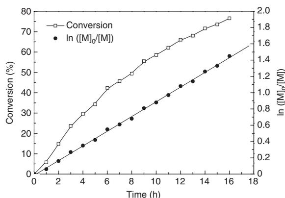
**Figure 1:** First order kinetics plot of the photoinduced Fe-mediated ICAR ATRP of MMA. Polymerization conditions: [MMA]<sub>0</sub>/[EBiB]<sub>0</sub>/[FeCl<sub>3</sub>·6H<sub>2</sub>O]<sub>0</sub>/[TMEDA]<sub>0</sub>/[AIBN]<sub>0</sub> was 500:1:0.1:0.2:0.3. Temperature: room temperature. Miniemulsion conditions:  $w_{Brij\ 98}=1.5 \text{ g}$ ,  $w_{HD}=1.8 \text{ g}$ .
