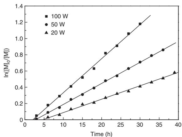
**Figure 3:** Kinetic plots of photoinduced Fe-mediated ICAR ATRP of MMA at different light intensities at 25°C. Temperature: 25°C. Miniemulsion conditions:  $w_{\text{Brij 98}}=1.5$  g,  $w_{\text{HD}}=1.8$  g.
