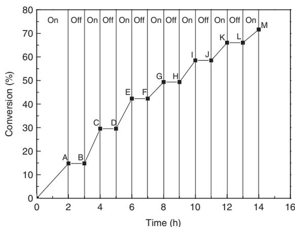
**Figure 5:** Photoinduced Fe-mediated ICAR ATRP of MMA at 25°C in the presence ("ON") or in the absence ("OFF") of light. Miniemulsion conditions:  $w_{\text{Brij 98}}=1.5$  g,  $w_{\text{HD}}=1.8$  g.
