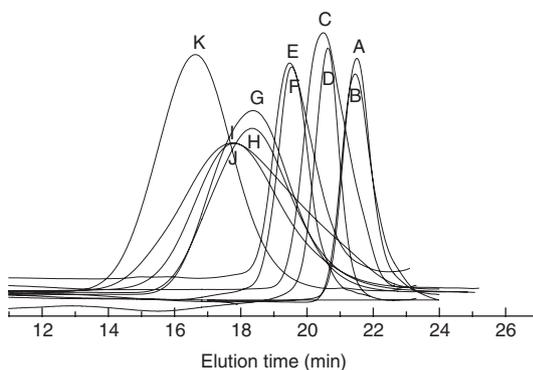
**Figure 6:** GPC curves of photoinduced Fe-mediated ICAR ATRP of MMA at 25°C. The polymerization conditions were the same as Figure 5.
