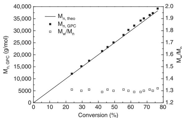
**Figure 2:** Plots of  $M_{n,GPC}$  and molecular weight distribution (MWD) versus percentage monomer conversion for the photoinduced Fe-mediated ICAR ATRP of MMA at 25°C in miniemulsion. The polymerization conditions were the same as Figure 1.
