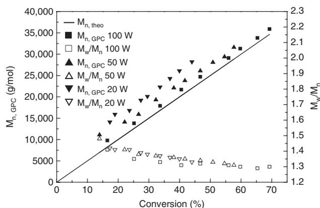
**Figure 4:** The molecular weight and molecular weight distribution of resulting polymers photoinduced Fe-mediated ICAR ATRP of MMA as a function of conversion. The polymerization conditions were the same as Figure 3.
