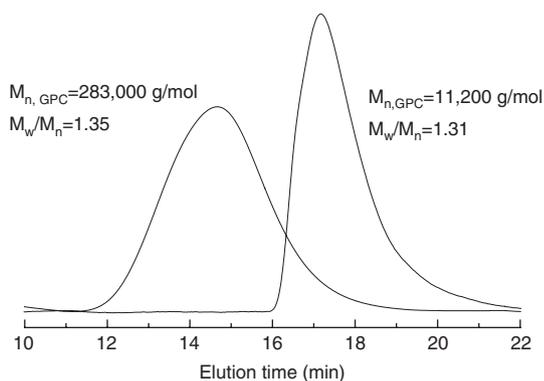
Figure 8: GPC traces of the macroinitiator PMMA-Cl ( $M_{n,GPC}=11,200$  g/mol,  $M_w/M_n=1.31$ ) and the chain extended PMMA ( $M_{n,GPC}=28,300$  g/mol,  $M_w/M_n=1.35$ ).
