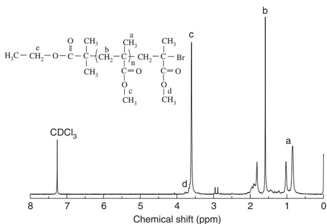
Figure 7:  $^1H$  NMR spectrum of PMMA-Cl.
