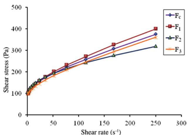
**Figure 2:** Rheograms representing the rapid viscosity profiles of hydrogels.
