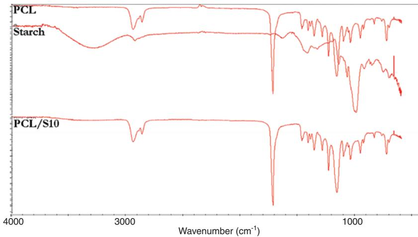
**Figure 4:** FTIR spectra of polycaprolactone, starch, and PCL/S10 composite.
