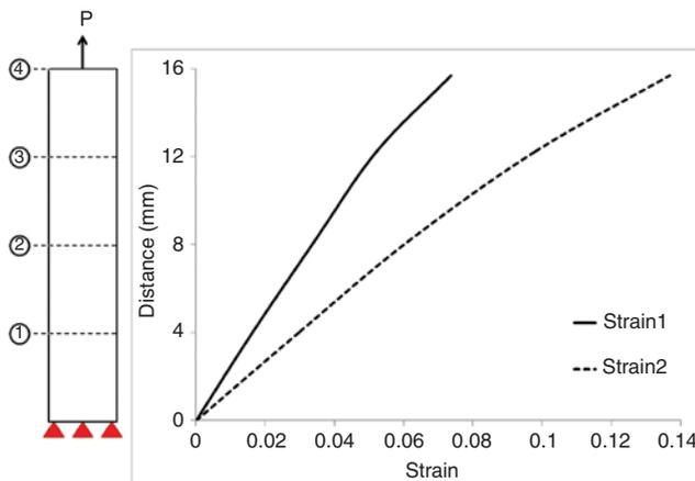
**Figure 6:** Schematic of tensile specimen and the measured strain at various points.
