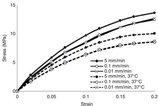
Figure 3: Stress-strain curves of PCL/starch composite at various strain rates measured at 23°C and 37°C.
