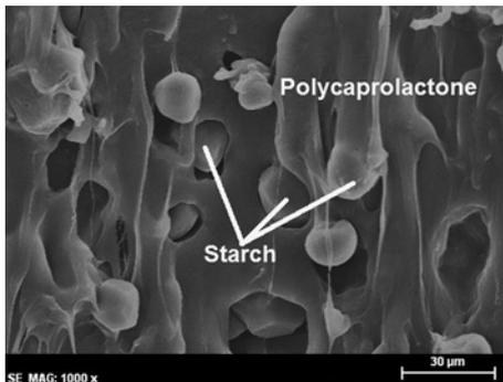
Figure 2: Morphology of PCL/S10 composite cross section.
