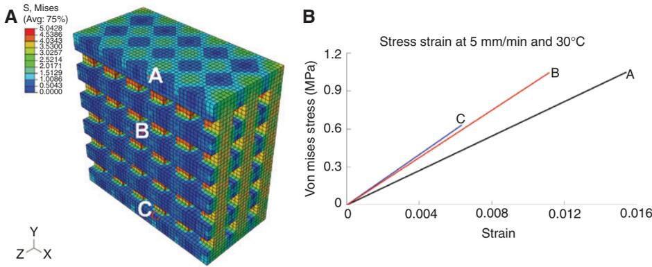
**Figure 7:** (A) Stress distribution within in the loaded PCL/starch composite scaffold model at its cross section and (B) stress-strain curves at three points across the scaffold.
