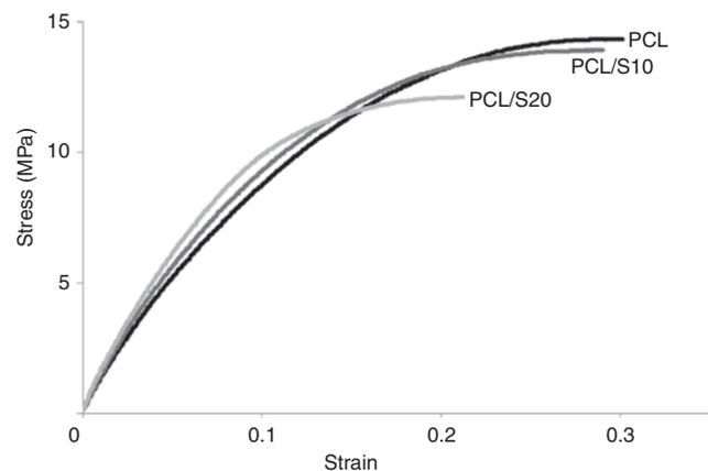
**Figure 1:** Typical stress-strain curves for PCL and its starch composites.
