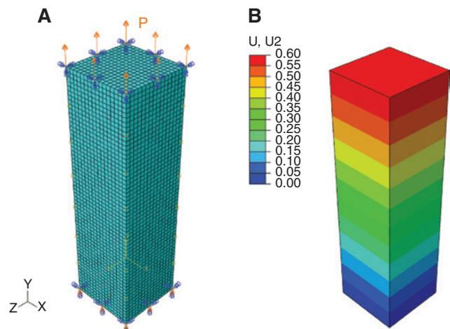
**Figure 5:** (A) Tensile test specimen with boundary conditions and loading P shown and (B) strain (in Y direction U2) distribution within the tensile specimen loaded at 5 mm/min at 30°C.
