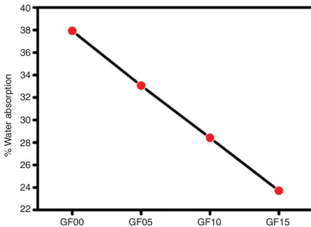
Figure 5: Water absorption of RPUGF vs. glass fiber quantity.
