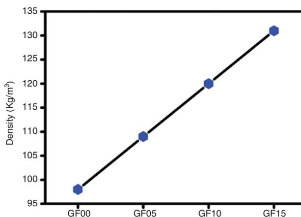
**Figure 1:** Density of RPUGF vs. glass fiber quantity.
