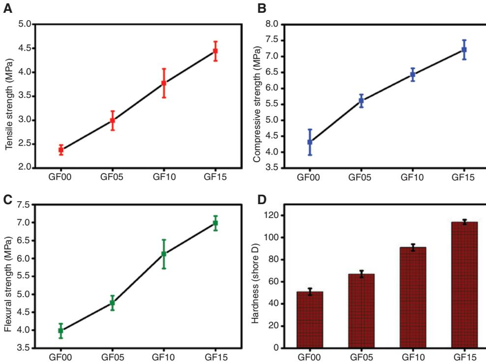
Figure 4: Mechanical properties of RPUGF vs. glass fiber quantity.
