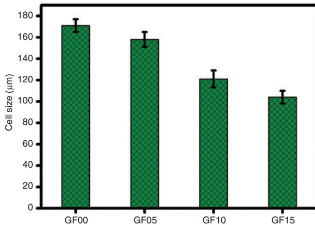
Figure 3: Cell size of RPUGF vs. glass fiber quantity.
