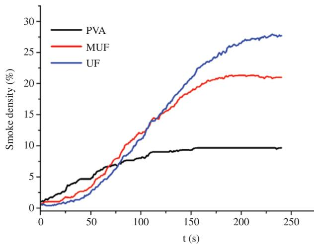
Figure 1: Smoke density of different composite materials.
