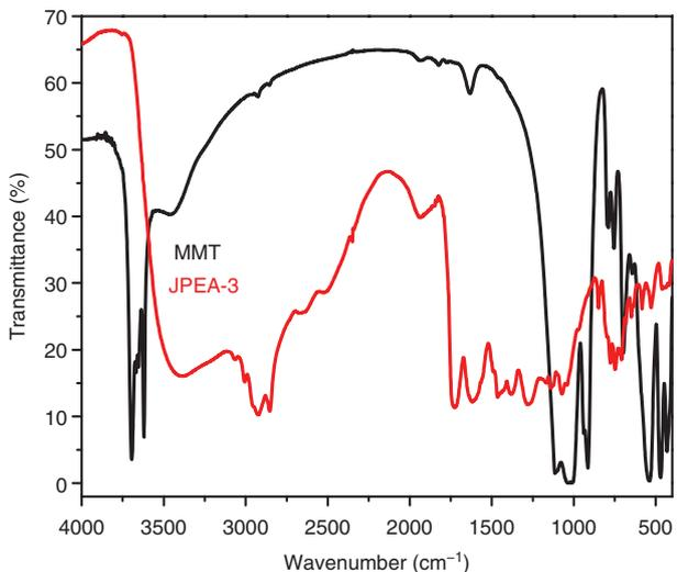
Figure 2: FTIR spectra of pure MMT and JPEA-3.
