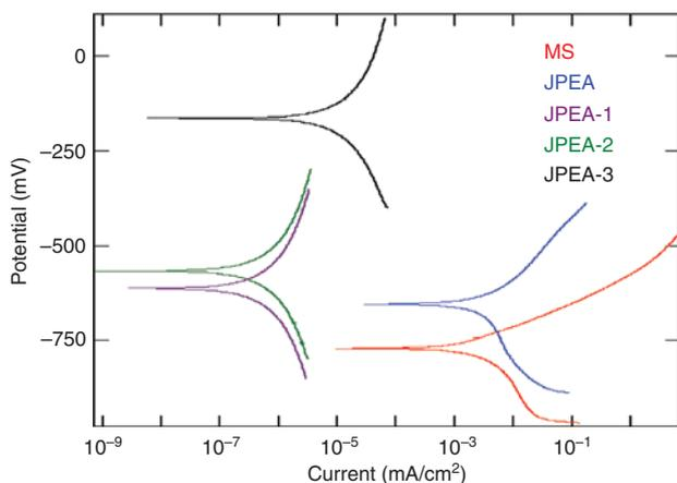
**Figure 9:** Tafel graph of bare MS and JPEA coated MS in 3.5% NaCl.
