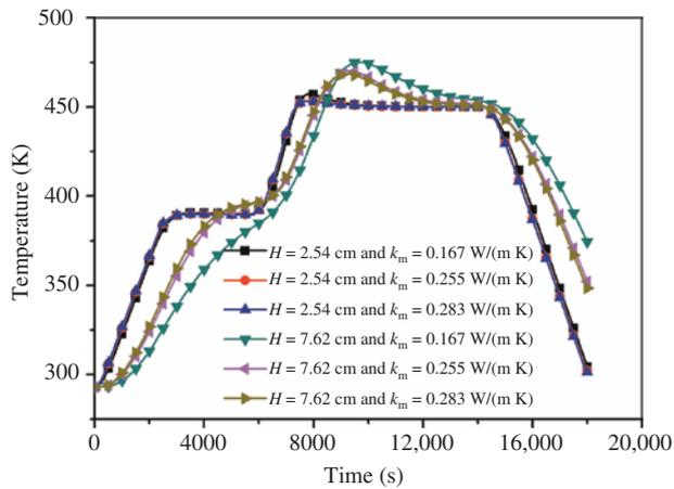
**Figure 6:** Development of temperature at central point of laminate with different conductivity coefficients.
