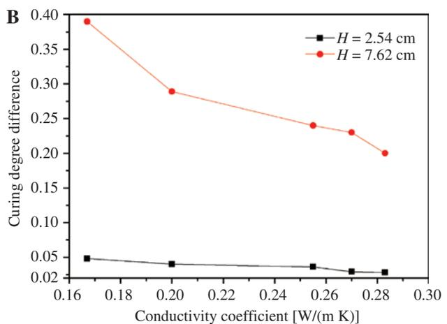
**Figure 8:** Effects of conductivity coefficient on curing uniformity: (A) temperature difference vs. conductivity coefficient, (B) curing degree difference vs. conductivity coefficient.
