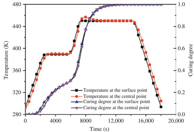
**Figure 2:** Comparison of the temperature and curing degree of the surface and central points for 2.54 cm plate.
