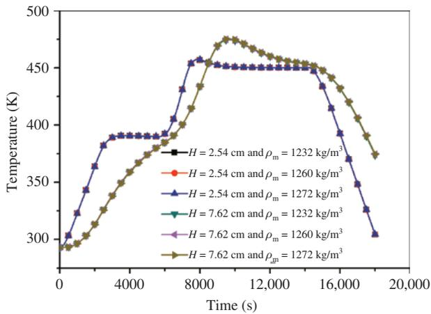
**Figure 3:** Development of temperature at central point of laminate with different densities of resin.
