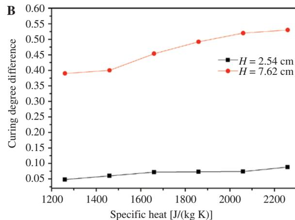
**Figure 11:** Effects of specific heat on curing uniformity: (A) temperature difference vs. specific heat, (B) curing degree difference vs. specific heat.
