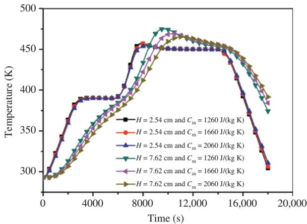
**Figure 9:** Development of temperature at central point of laminate with different specific heat capacities.
