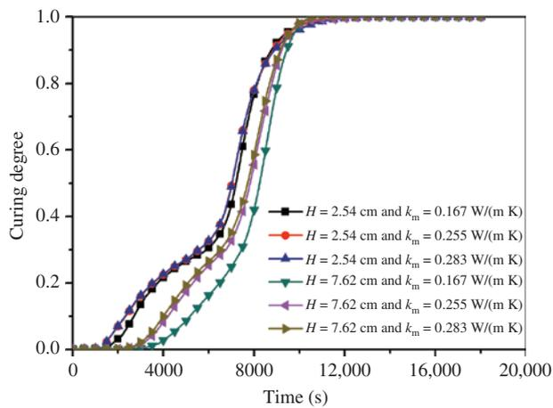
**Figure 7:** Development of curing degree at central point of laminate with different conductivity coefficients.
