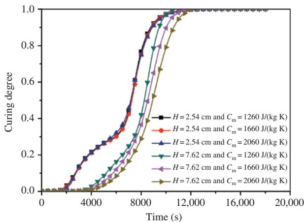
**Figure 10:** Development of curing degree at central point of laminate with different specific heat capacities.
