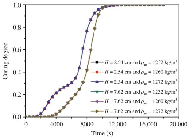
**Figure 4:** Development of curing degree at central point of laminate with different densities of resin.
