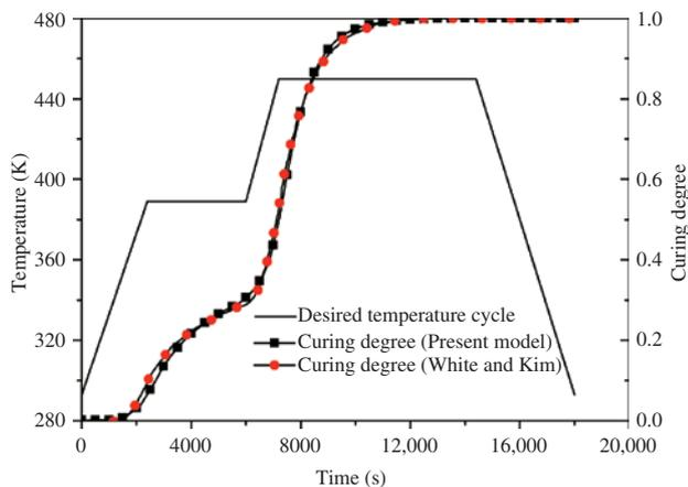
**Figure 1:** Desired temperature cycle and comparison of the curing degree at the central point between the present model and the previous model.
