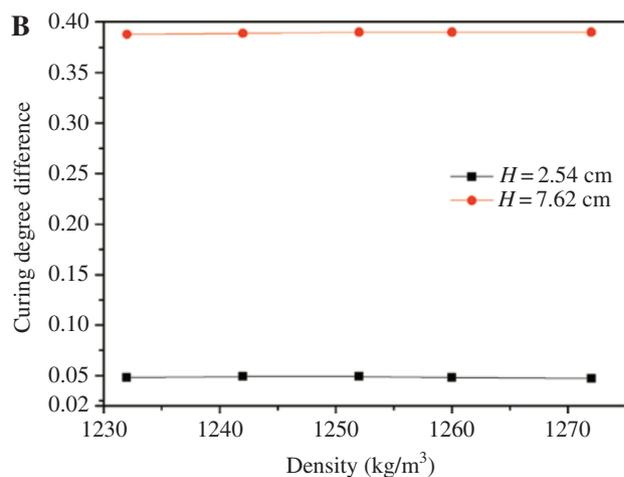
**Figure 5:** Effects of density on curing uniformity: (A) temperature difference vs. density, (B) curing degree difference vs. density.
