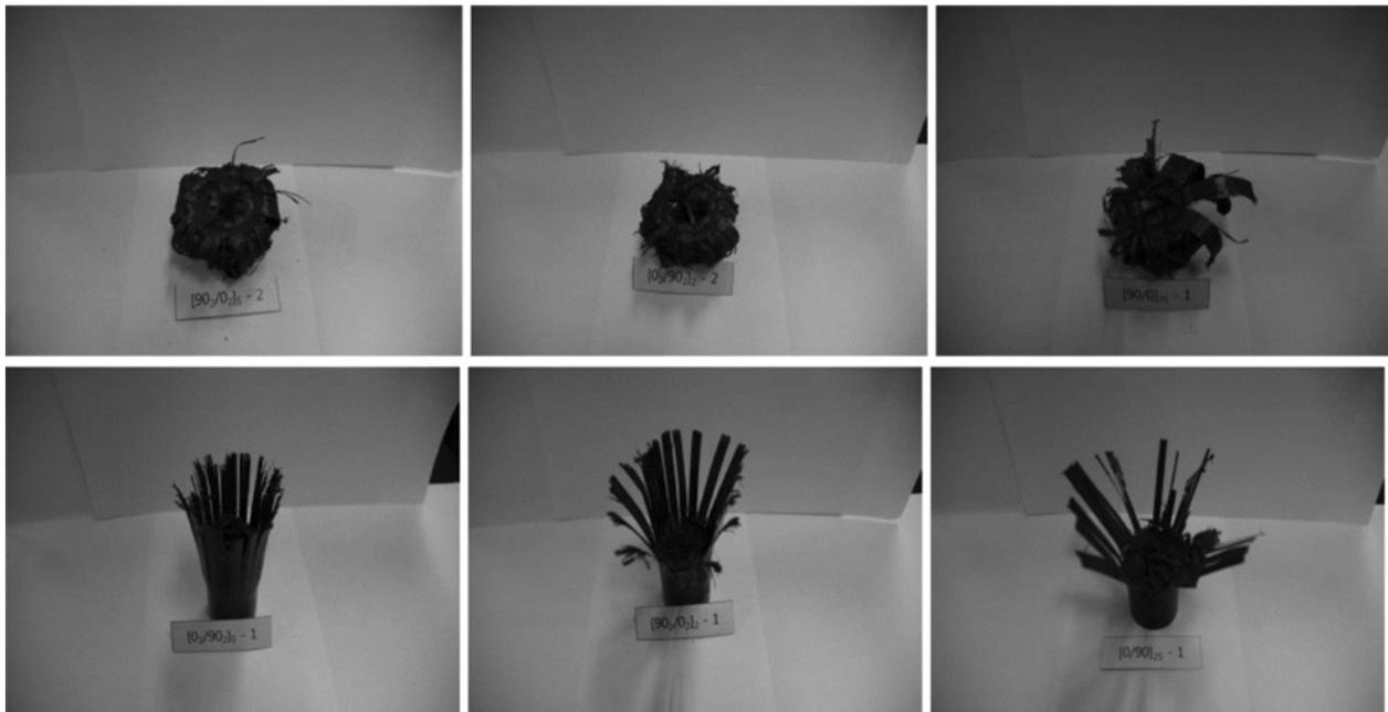
Figure 5: Typical collapse modes of the 90° external sheet CFRP specimen and typical collapse modes of the 0° external sheet CFRP specimens.
