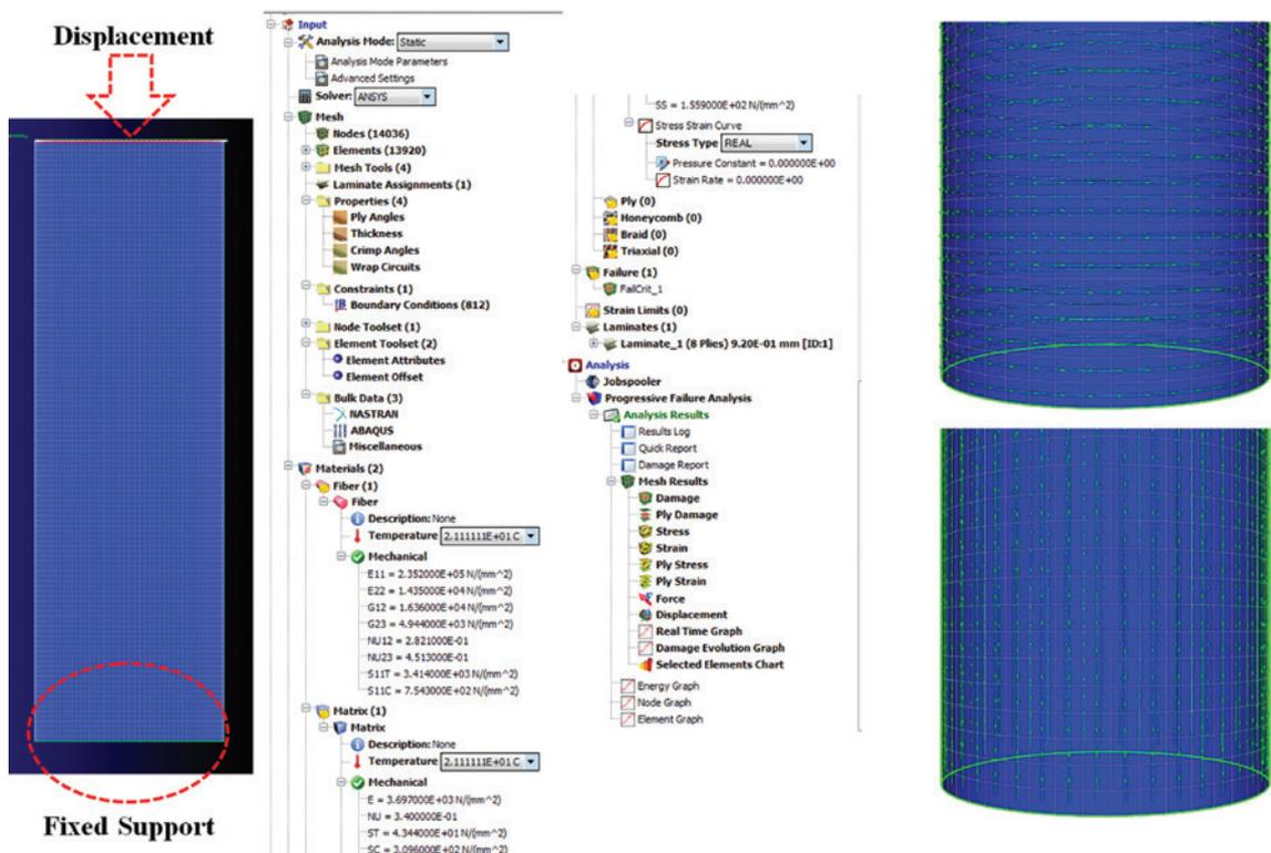
Figure 4: Boundary condition setting and GENOA analysis process and fiber direction according to the external stacking angle changed.
