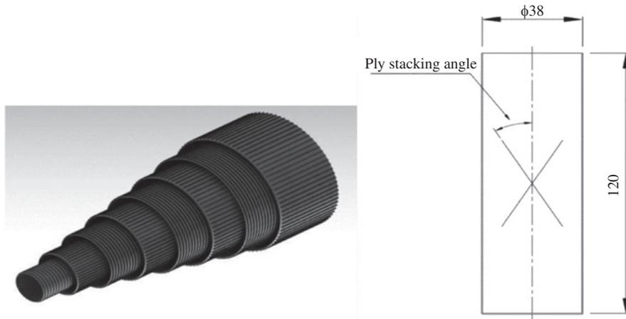
Figure 1: Static collapse specimen circular member geometry and drafting.
