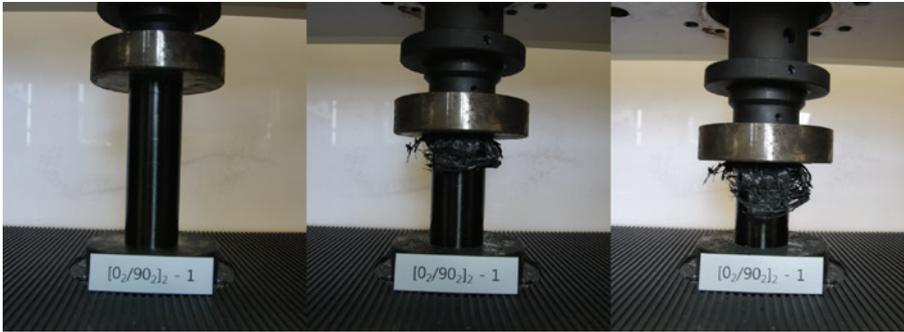
Figure 2: Collapse processing of a circular CFRP composite structure member,  $[90_2/0_2]_5$ .
