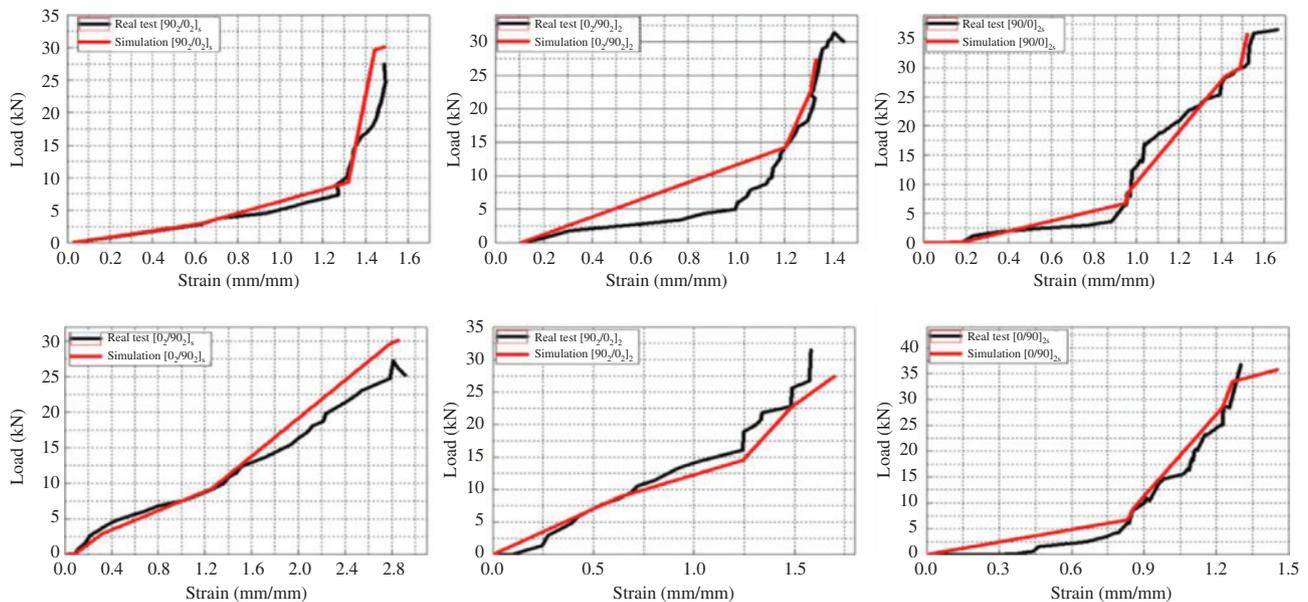
Figure 7: Comparisons between the experimental and simulation load-displacement curves collapse-test results for specimens  $[90_2/0_2]_1$ ,  $[0_2/90_2]_1$ ,  $[90/0]_{2s}$ ,  $[0_2/90_2]_1$ ,  $[90_2/0_2]_2$  and  $[0/90]_{2s}$ .
