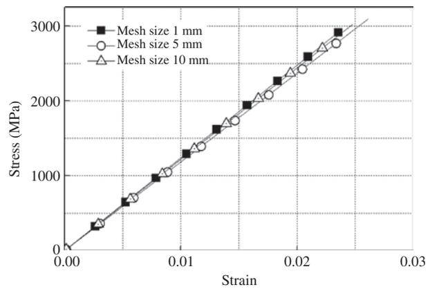
Figure 3: Grid independence test on  $[\pm 0]_{10}$  tensile testing.
