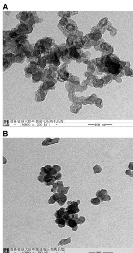
Figure 1: TEM images of C-CB and I-CB particles. (A) C-CB and (B) I-CB.
