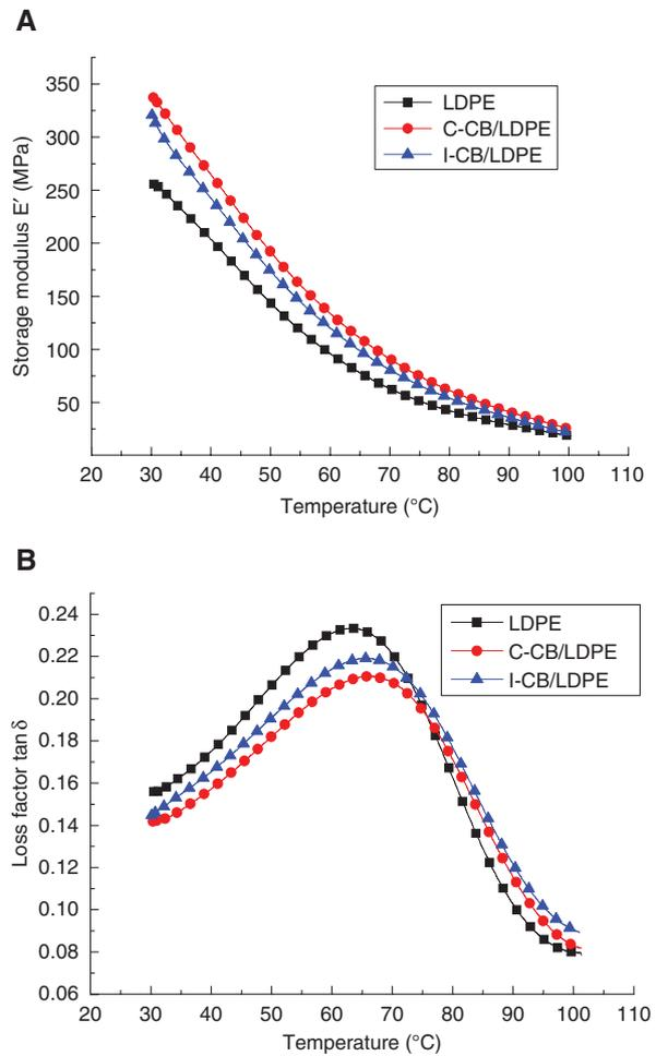
**Figure 6:** Temperature dependence of  $E'$  and  $\tan \delta$  for LDPE and the CB/LDPE nanocomposites.
