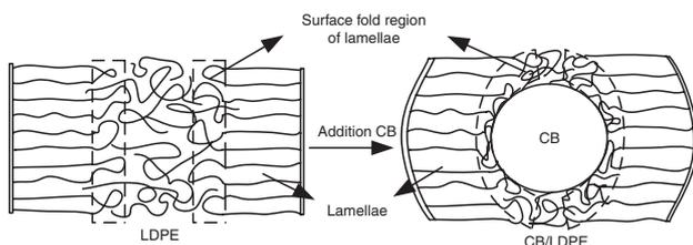
**Figure 9:** Effect of CB particle in the amorphous phase between lamellae crystals.
