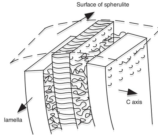
Figure 8: Diagram of spherulite structure for polyethylene.
