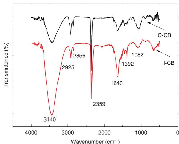
Figure 2: FTIR spectra of C-CB and I-CB.
