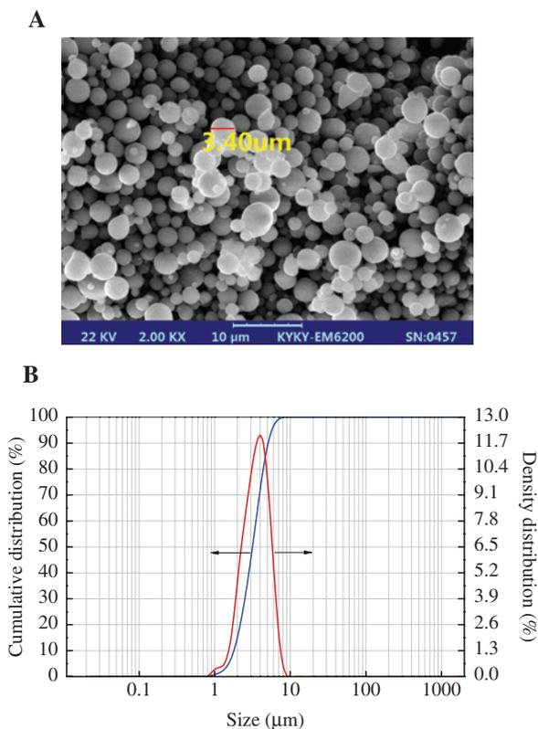
**Figure 1:** Micron-aluminum particles of (A) SEM image and (B) particle size distribution graph.
