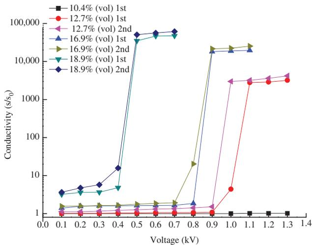
**Figure 4:** Conductivity-voltage curve of ER/MP.
