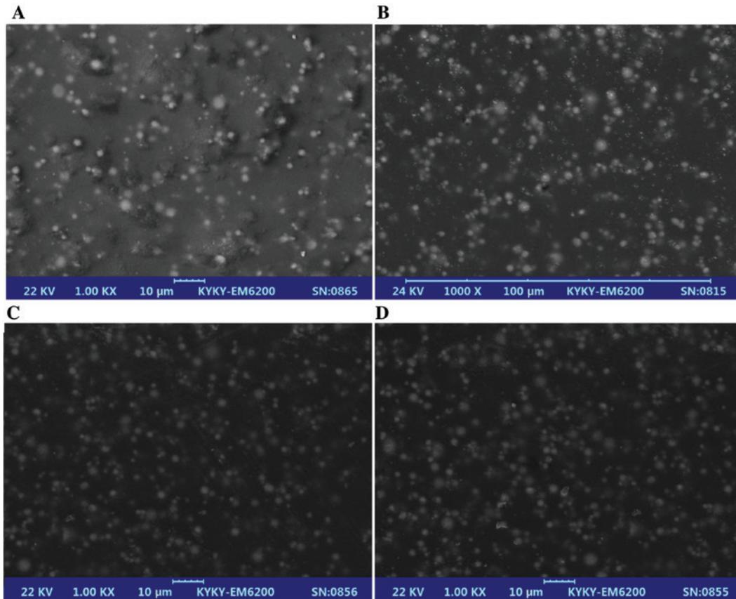
**Figure 3:** SEM images of ER/MP composites: (A) volume concentration of 10.5%, (B) volume concentration of 12.7%, (C) volume concentration of 16.9% and (D) volume concentration of 18.9%.
