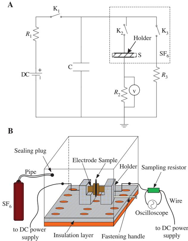
**Figure 2:** Measuring circuit and experimental setup. (A) Circuit for conductivity under applied voltage:  $R_1$ -current limiting resistor,  $R_2$ -sampling resistor,  $R_3$ -discharge resistor,  $S$ -sample and DC-regulated power supply and (B) experimental setup.
