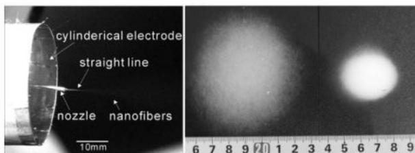
**Figure 5:** Cylindrical electrode used to stabilize electrospun fibers. a) Nanofibers with an auxiliary electrode surrounding the nozzle. b) Deposition of fibers without an aux. field c) Deposition of fibers with an aux. field. Shown units are in centimeters. The size of the deposition area is reduced with the application of an auxiliary electrical field. Reprinted with permission from G.H. Kim [80]. Copyright 2006 John Wiley and Sons.
