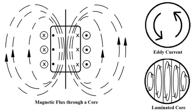
**Figure 8:** Magnetic flux and eddy current visualization through core (side and bottom). The eddy current causes a decrease in magnitude of the magnetic field. Laminating the core prevents this effect.
