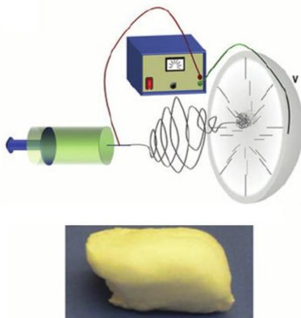
**Figure 12:** Creation of the Focused, Low density, Uncompressed nanofiber (FLUF). Top: FLUF electrospinning setup using a plastic hemisphere with grounded needles placed at regular intervals throughout the interior to collect the fibers; Bottom: finished FLUF scaffold. Modified and reprinted with permission. Copyright © 2011 Elsevier Publishing [155].
