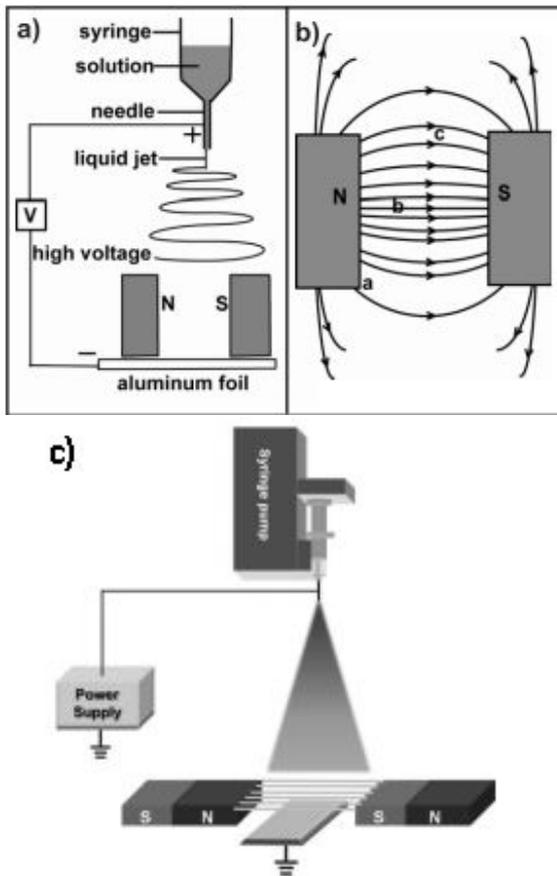
**Figure 7:** Alignment of electrospun fibers using magnetism [111, 112]. In both examples, two permanent magnets were used to collect parallel nanofibers on the target.
