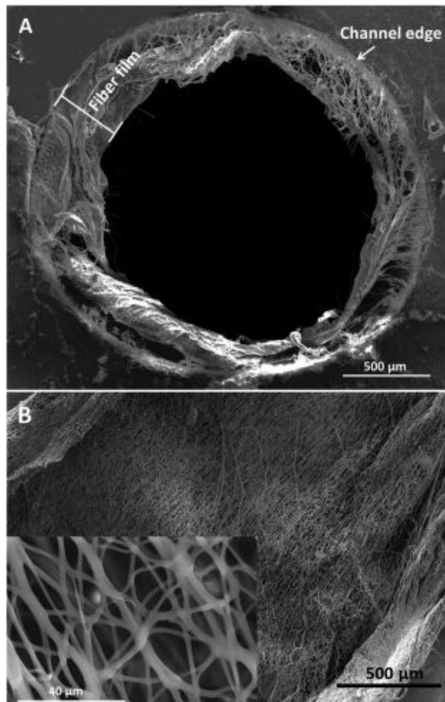
**Figure 10:** SEM images of a fiber coated channel looking A) through the opening and B) along the channel. Reprinted with permission from Chen *et al.* [124]. Copyright 2016 The Royal Society of Chemistry.
