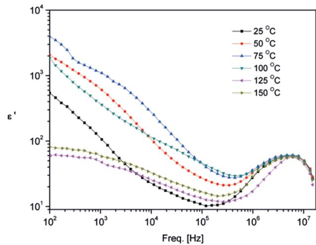
Fig. 2: Frequency dependency of the real part of dielectric constant at different temperatures.
