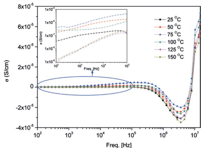
Fig. 6: Frequency dependence of the real part of conductivity at different temperatures.
