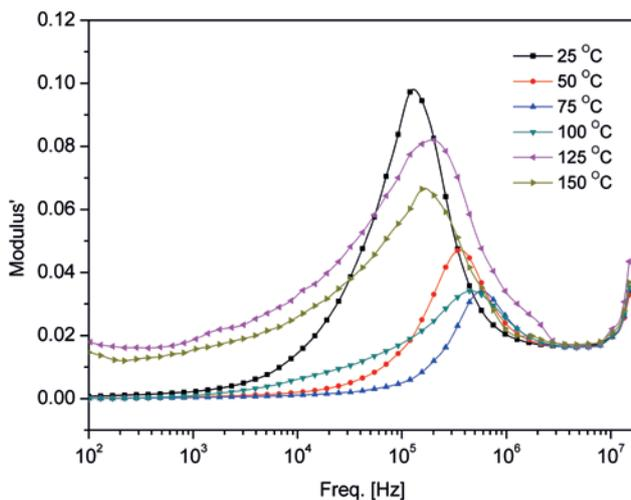
Fig. 4: Frequency dependence of  $M'$  at various temperatures.
