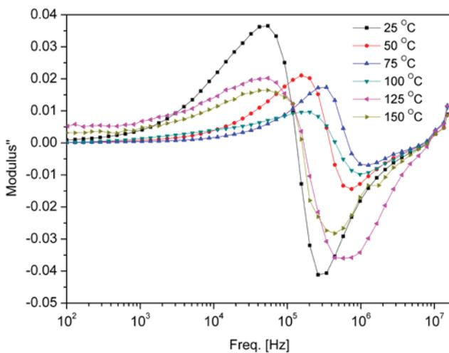
Fig. 5: Frequency dependence of  $M''$  at various temperatures.
