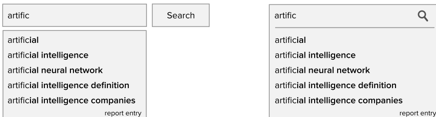
Figure 1: The figure shows the wireframes of textual autocompletion in the special case of query autocompletion. Both versions offer the same functionality. They make partial user input more complete. On the left: A user interface composed of three components, an input field, a suggestion area, and a button for confirmation. With loose interface elements. On the right: A more compact version with adapted visual composition. The search button was replaced by an icon of a magnifying glass. The search field and the suggestion area are combined into one field. Both examples show an option in the bottom right of the suggestion area to report inappropriate entries.
