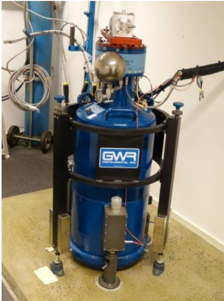
**Figure 5:** Superconducting gravimeter GWR#54 at Onsala Space Observatory.
