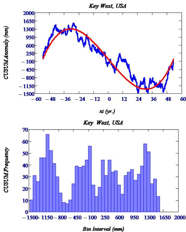
Fig. 5. Residuals and the estimated uniform acceleration's CUSUM charts at Key West, USA, TG station (top). The histogram of the residuals compartmentalizes the residuals before and after the critical points and the inflection point.
