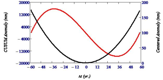
**Fig. 1.** The graph is intended to show the discernable properties of the CUSUM of a uniform acceleration and its magnification (referenced to the two different vertical axes for clarity). Parabolic behaviour of a centered sea level anomaly due to a uniform acceleration  $a = 0.10$  mm/yr. is shown in *black* and referenced to the right vertical axis. Its CUSUM, shown in *red*, is referenced to the left vertical axis.
