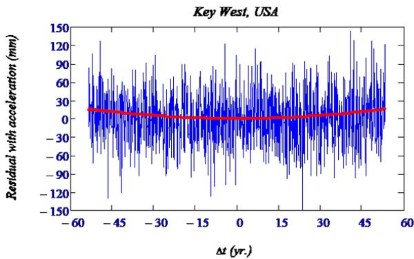
**Fig. 3.** The unmodeled uniform acceleration, shown in red, is embedded in the residuals, which is difficult to discern and verify if it is uniform.
