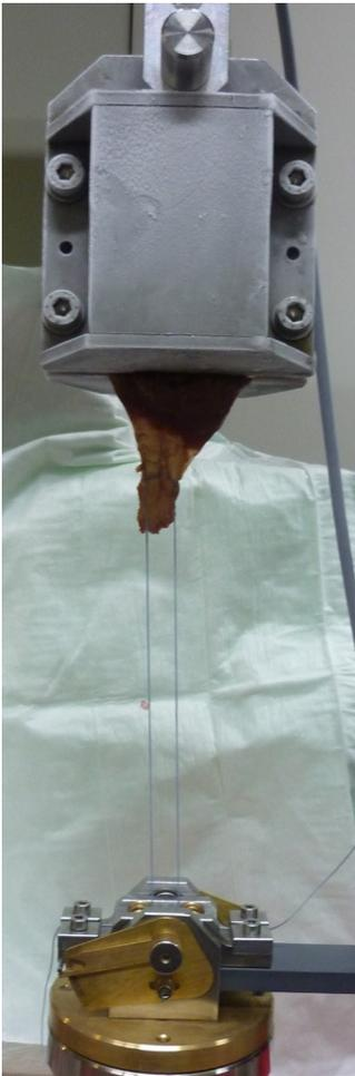
**Figure 3:** Part of the Zwick UTM test setup. DLKS is shown. The infraspinatus muscle is clamped using two metal brackets of a cryo-jaw (upper part of the picture). The compensator device is mounted on the UTM base (lower part of the picture).
