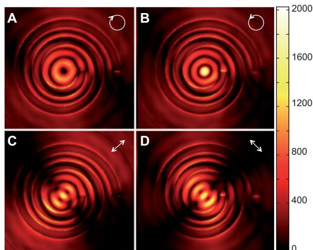
**Figure 4** Simulation of the electric field distribution at the surface of an Au film patterned with an RH spiral groove and air. The spiral groove is illuminated with (A) RHCP, (B) LHCP, and (C, D) two orthogonal linearly polarized Gaussian beams at 830 nm. The direction of propagation of the beam is normal to the patterned metal surface.
