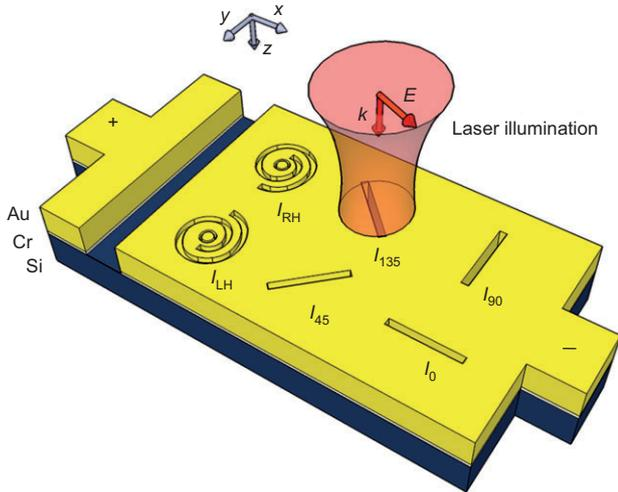
**Figure 1** Schematic diagram of the proposed plasmonic polarimeter that consists of six, differently shaped plasmonic slit structures patterned into an Au film on top of a Si-based Schottky detector. Photocurrent measurements on different plasmonic structures enable a direct determination of the state of polarization of an incident light beam.
