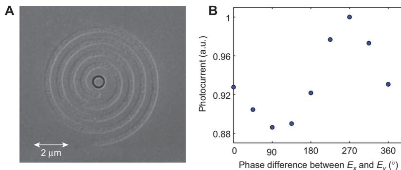
**Figure 5** (A) SEM image of a coaxial aperture surrounded by an RH spiral groove fabricated with FIB. (B) Normalized measured photocurrent of the coaxial aperture shown in (A) as a function of the phase difference between  $E_x$  and  $E_y$ .
